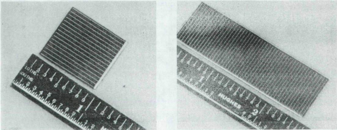
Figure 1. - High efficiency solar cells.
