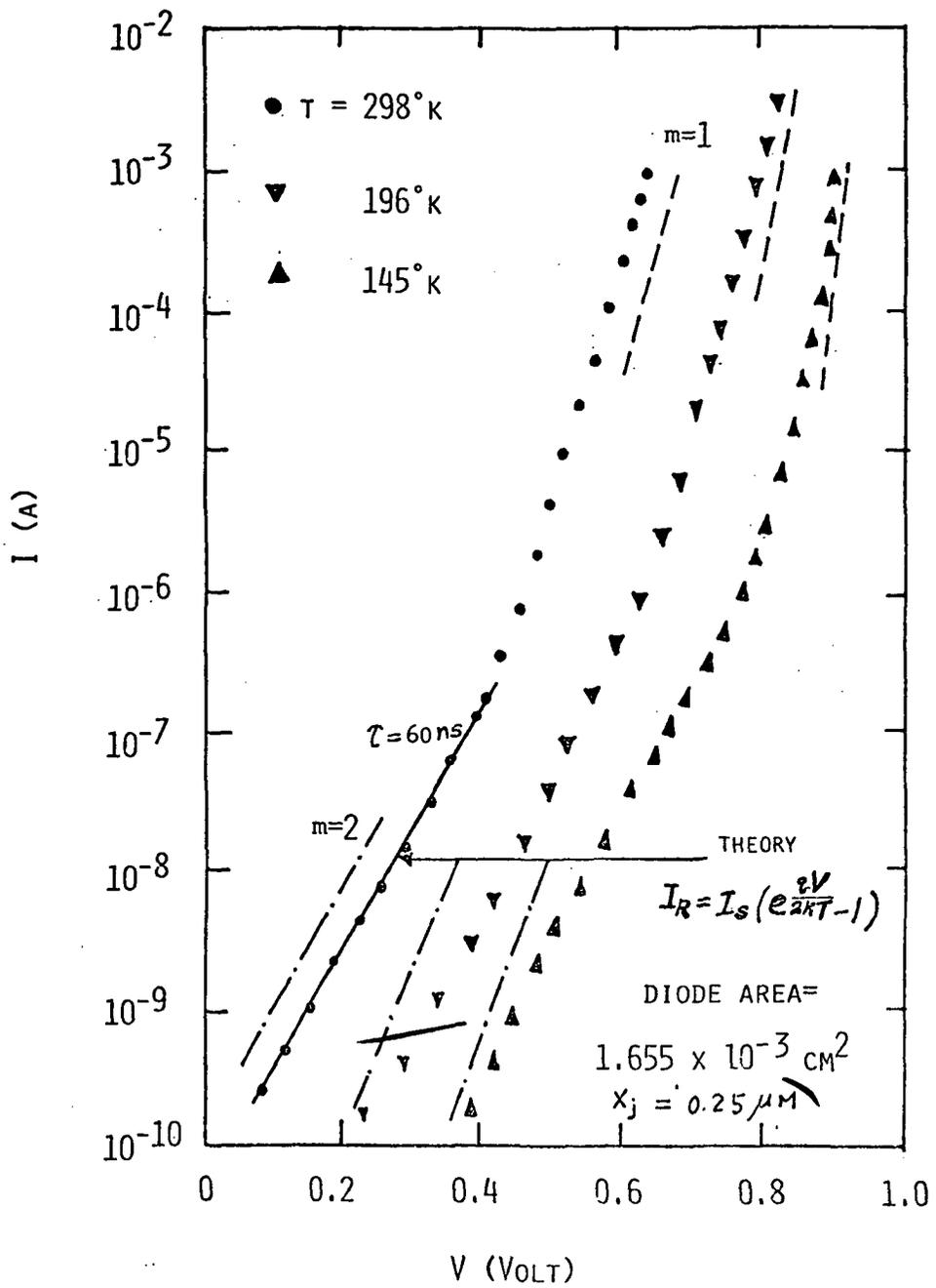
Figure 1. - I - V characteristics for a 0.1 ohm-cm silicon N<sup>+</sup>-P junction solar cell.
