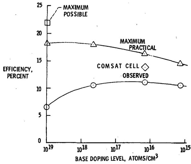
Figure 1. - Calculated efficiencies of silicon solar cells.
