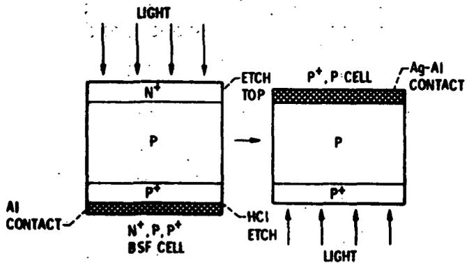
Figure 1. - Fabrication of  $p^+, p$  cells.
