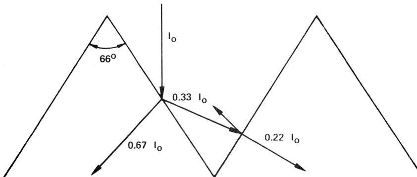
Figure 3 - Optical path schematic of CNR tetrahedral surface.
