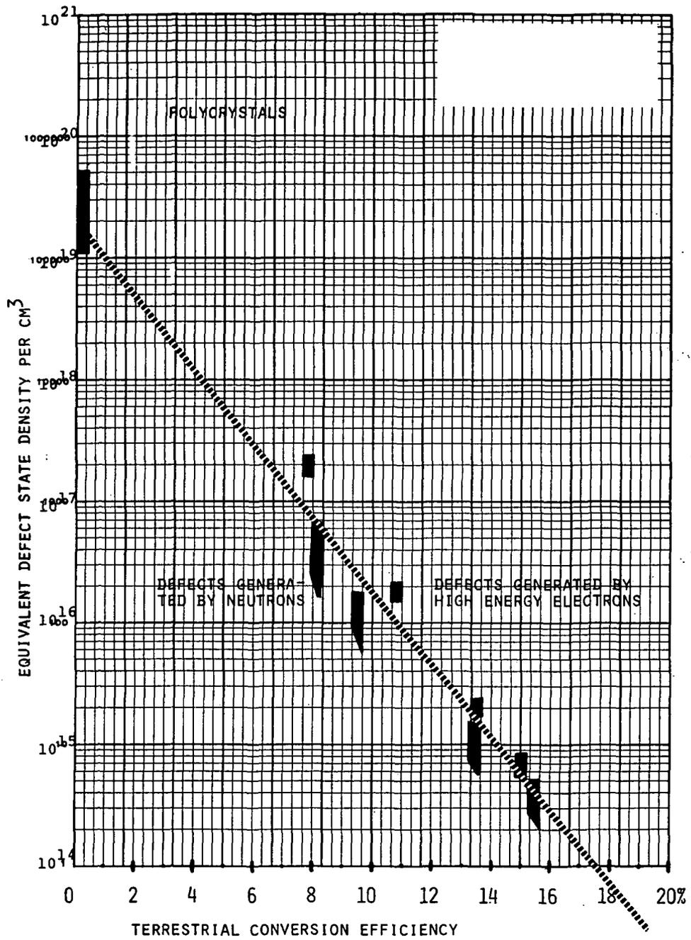
Figure 3. - Crystallographic order requirements for efficient conversion.
