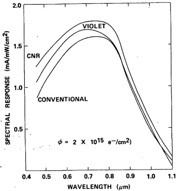
Figure 10. - Relative spectral response of CNR, violet, and conventional cells after a fluence of  $2 \times 10^{15} \text{ e}^-/\text{cm}^2$ .
