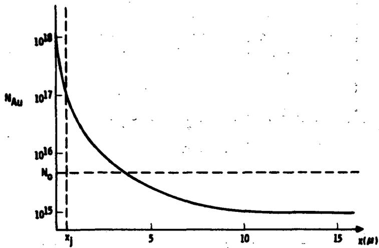
Figure 7. - Gettering of deep impurities by diffusion process and possible distribution at junction.
