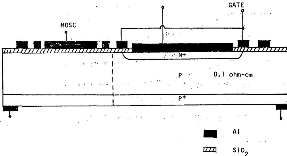
Figure 2. - Cross-sectional view of a silicon N<sup>+</sup>P diode with MOS guard ring gate, and a MOS capacitor.
