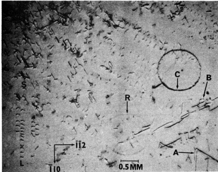
Figure 3. - A  $(\bar{2}20)$  topograph of the same region after 2 minute diffusion treatment in phosphorous oxychloride at  $1100^{\circ}\text{C}$ . Circular defects at C and R may be similar to electrically "dead" areas seen in commercial cells by scanning electron microscopy. Some dislocations, as at A and B, are visible in both topographs. Many dislocations are introduced by slip during this processing step, as at S-L. Magnification 16.9X. (L-89-LP104)
