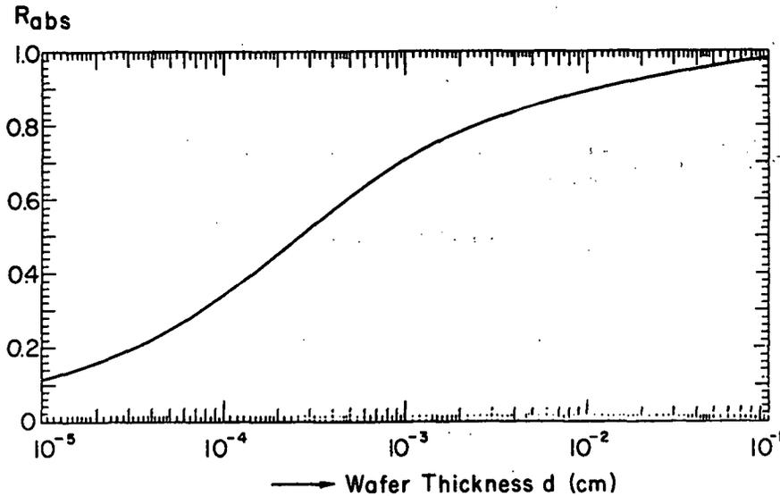
Figure 1. - Ratio  $R_{abs}$  of the number of photons absorbed in a single pass through a silicon layer of thickness  $d$  to the number entering the layer, as contained in airmass zero sunlight up to  $1.125 \mu\text{m}$  wavelength.  $T = 300^\circ \text{K}$ .
