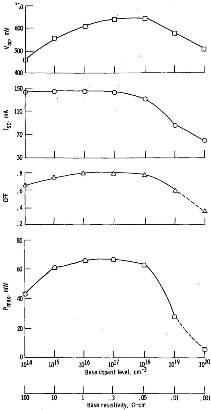
Figure 1. - Cell performance as function of base resistivity.
