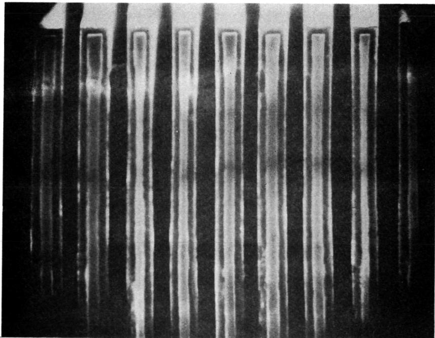
Figure 5. - Photomicrograph of grooved cell after antimony diffusion.
