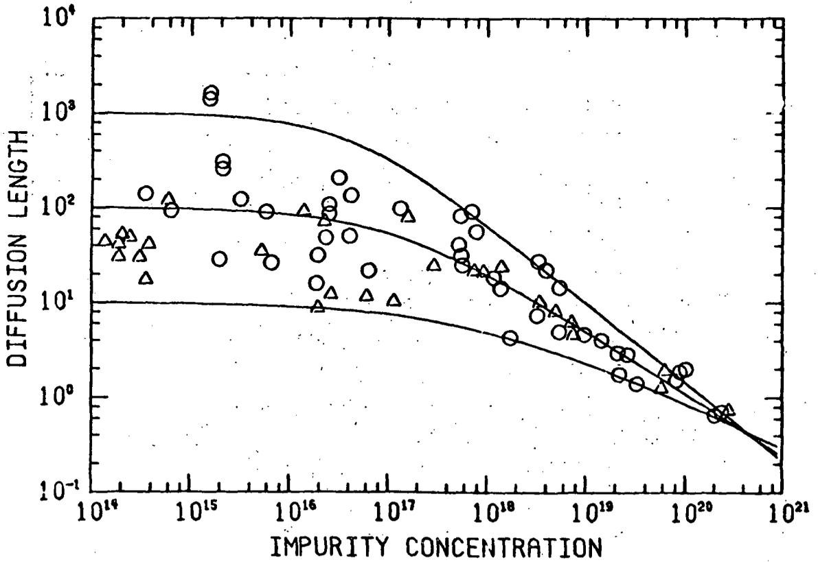
Figure 3. - Variation of diffusion length with impurity concentration.
