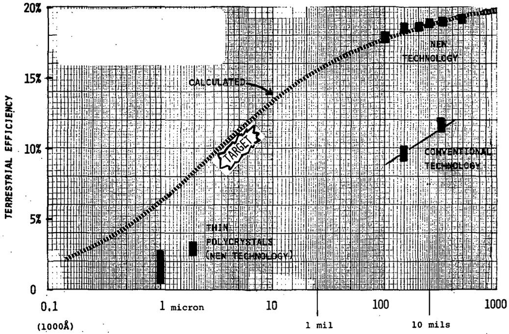
Figure 2 - Maximum efficiency as function of thickness.
