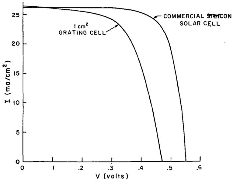
Figure 16. - Characteristic under simulated AMO illumination.
