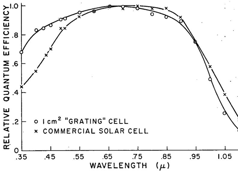
Figure 17. - Relative spectral response.
