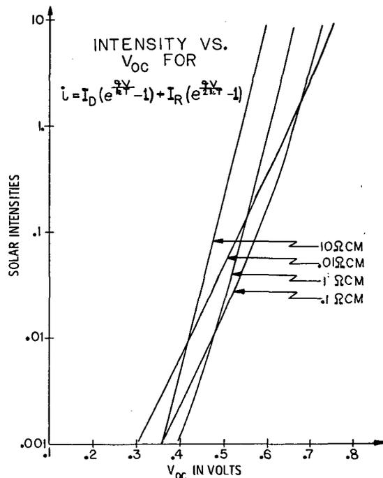
Figure 3. - Dependence of  $V_{oc}$  on solar intensities for generation-recombination limited solar cells with various base resistivities.
