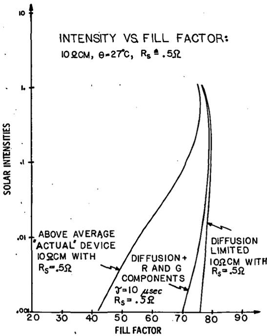
Figure 7. - Dependence of fill factor on solar intensities for solar cells with  $R_s = 0.5 \text{ ohm}$ .
