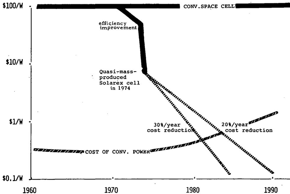
Figure 1. - Cost of solar cells as function of time at Solarex. Conventional space solar cells cost approximately \$100/W. Solarex has reduced the cost to levels below \$10/W in 1974. A continued cost reduction program is indicated by the 20% and 30%/year cost reduction lines. The cost of conventional power is intercepted between 1980 and 1990.
