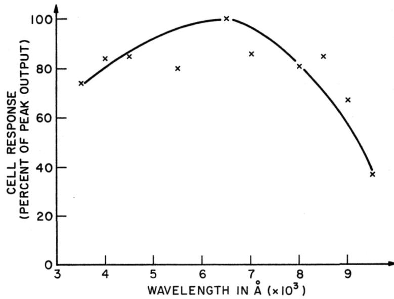
Figure 9. - Spectral response in metal/semiconductor cell.
