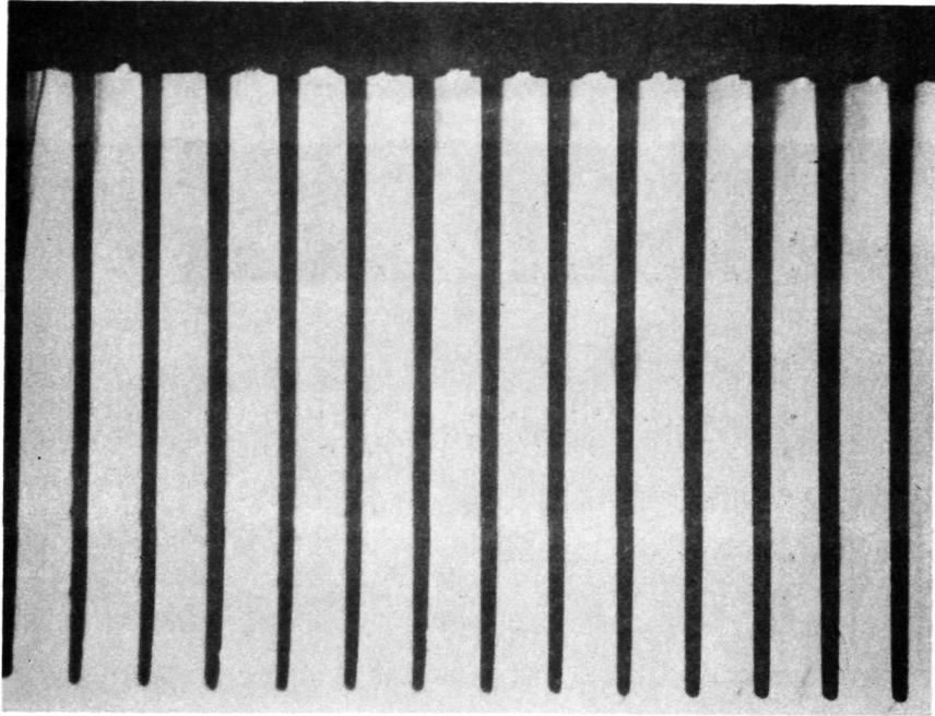
Figure 4. - Photomicrograph of 100- $\mu$ m-deep etched grooves.
