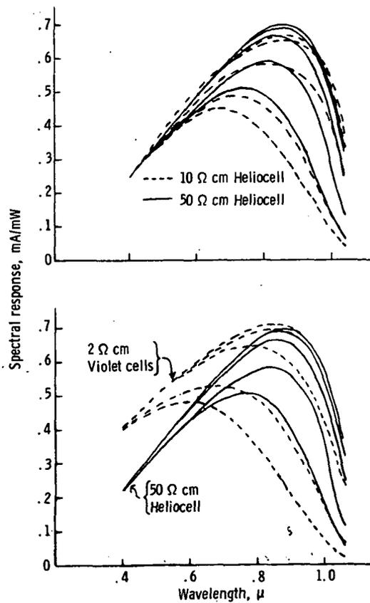
Figure 6. - Spectral response as function of wavelength.
