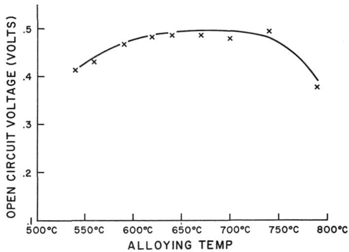
Figure 14. - Open circuit voltage versus alloying temperature.
