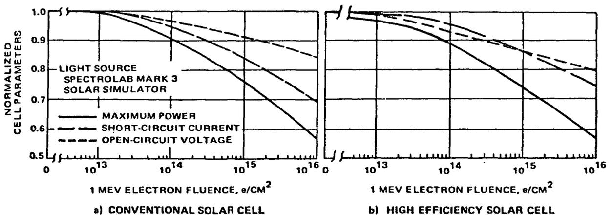
Figure 4. - High energy electron irradiation results.
