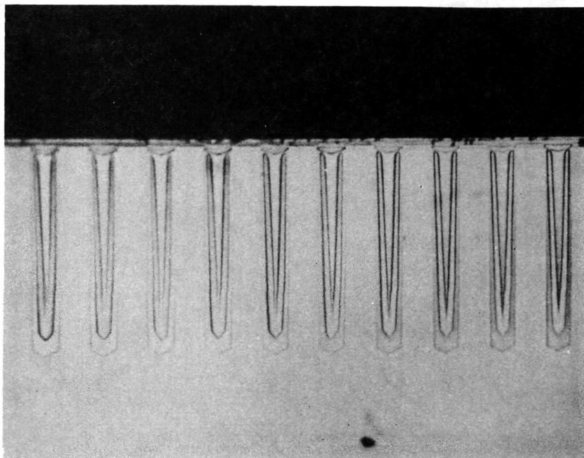
Figure 6. - Photomicrograph of grooved cell after epitaxial refill.
