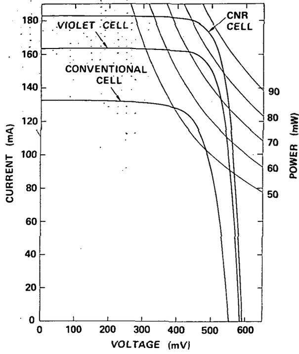
Figure 7. - Current-voltage characteristics of CNR, violet, and conventional cells under AMO illumination.
