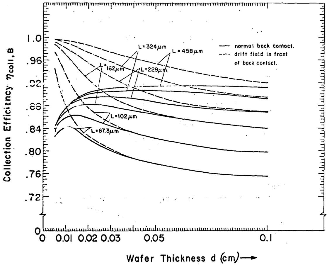
Figure 2. - Collection efficiency  $\eta_{coll,B}$  from the base region as function of wafer thickness  $d$ , for 3 values of diffusion length in the base region, with and without a drift field in front of the back contact. Airmass zero sunlight,  $T = 300^{\circ} K$ .  $x_{T,R} = 0.8 \mu m$ .
