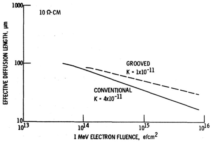
Figure 5. - Radiation damage of grooved solar cell.
