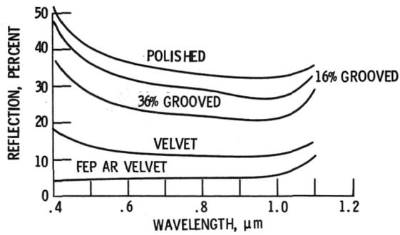
Figure 4. - Total reflection for various types of silicon surfaces.
