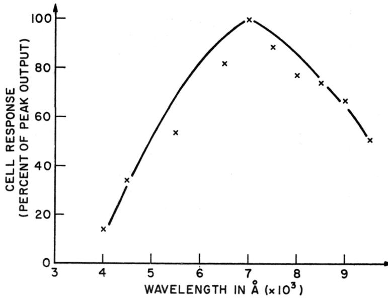
Figure 6. - Spectral response in area diffused cell.
