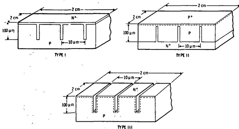
Figure 2. - Three designs for VMJ solar cells.
