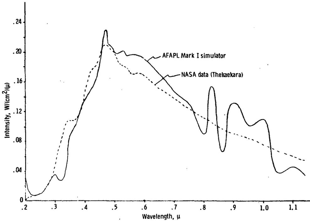
Figure 1. - Simulated and assumed AMO spectra.
