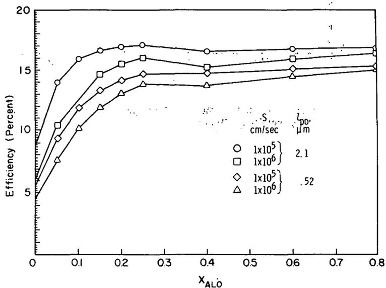
Figure 2. - Dependence of power conversion efficiency on  $X_{AL0}$ .
