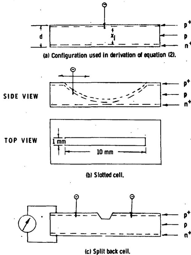
Figure 1. - Schematic diagrams of solar cell configurations.
