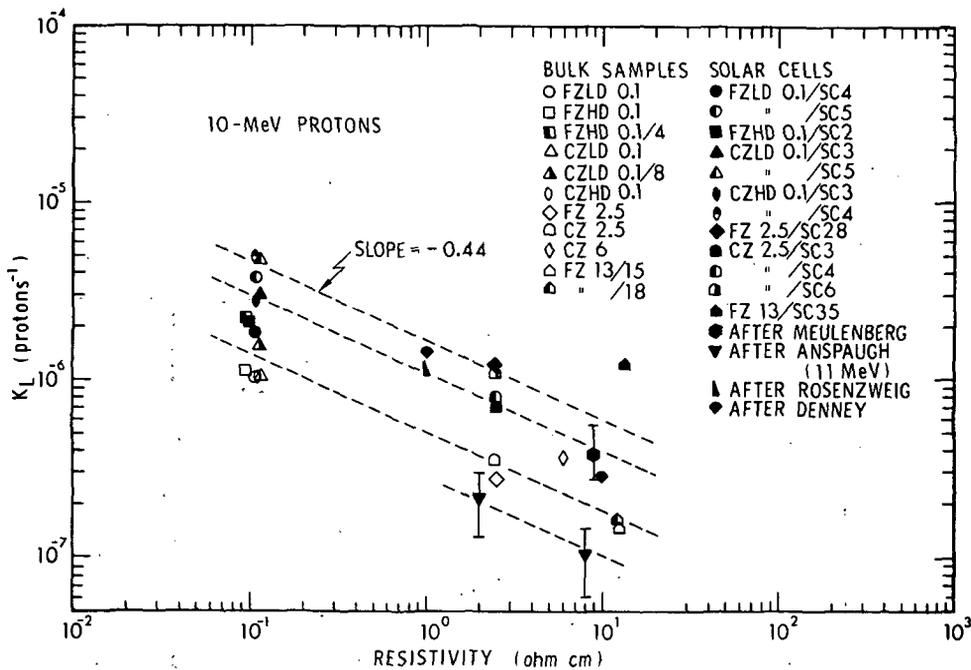
Figure 6. - Damage coefficient vs. resistivity for 10-MeV proton-irradiated bulk silicon specimens and silicon solar cells.
