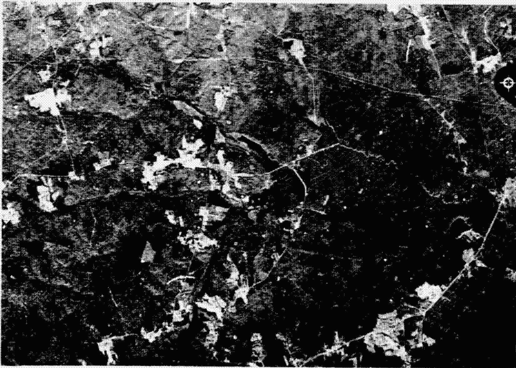
Figure 4.- U-2 photograph taken at 60,000 feet. Locations of 7 sections of Swift Creek Reservoir, used in checking precision and accuracy of area measurements from LANDSAT, are shown in Figure 5 and 6.
