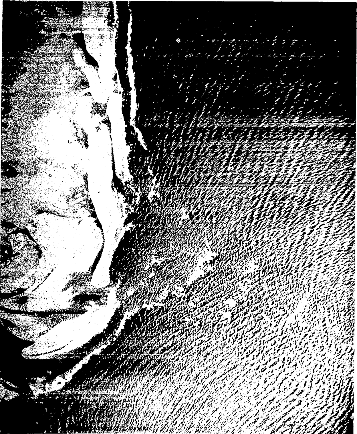
FIGURE 4.9 WAVE REFRACTION OVER SUBMARINE RIDGE SHOWING CROSSED WAVE PATTERNS.
