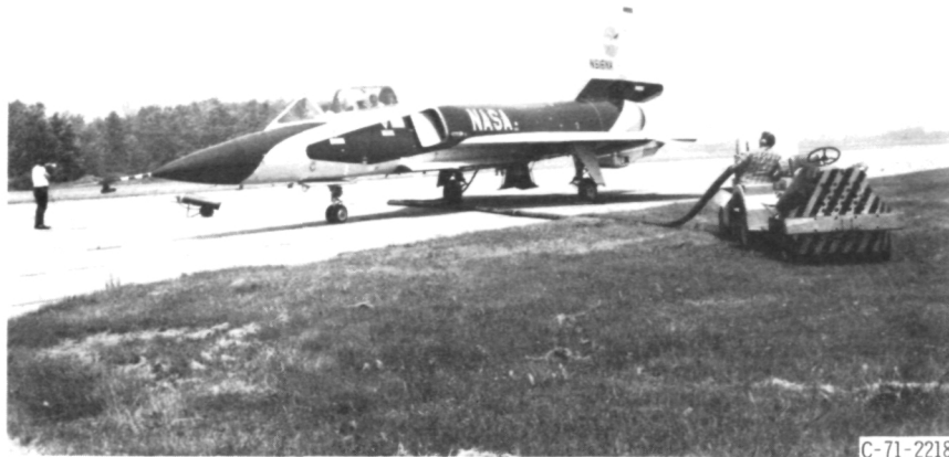
Figure 10. - Location of external source of cooling air for static tests.
