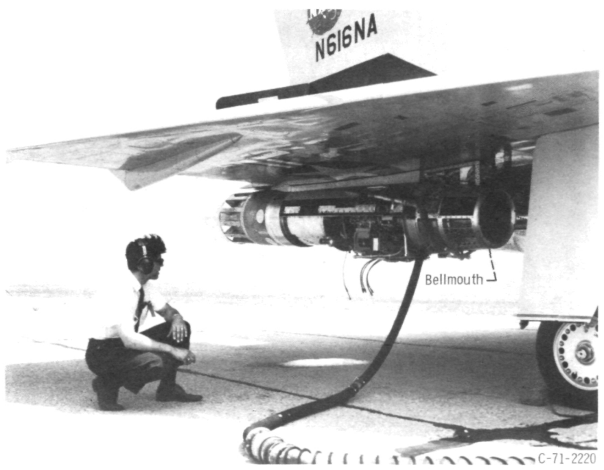
Figure 3. - Nacelle modification for static tests.
