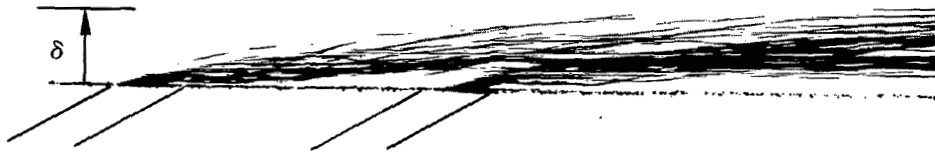
Figure 11. - Streaklines during injection into thick boundary layer at velocity ratio of 0.80.
