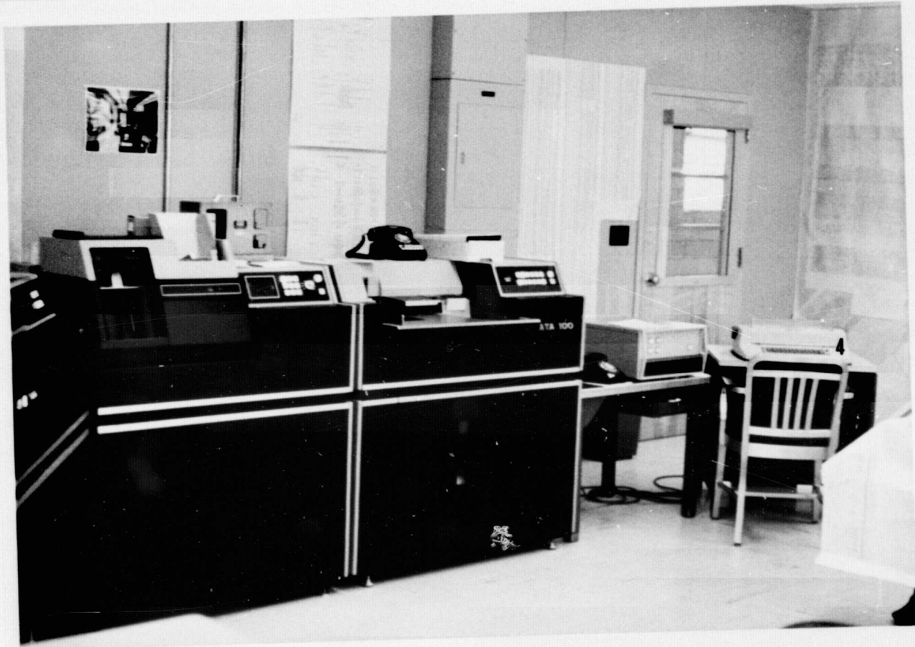
Fig. 9. The 2780 remote terminal located at Wallops Flight Center. (1) printer; (2) card reader; (3) card punch; (4) typewriter terminal (IBM 2741 Communications Terminal).
