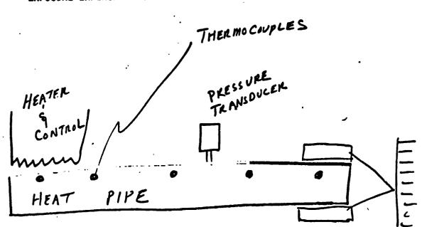
3.6 SKETCH EXPERIMENT INCLUDING MAJOR COMPONENTS AND LAYOUT FOR EXPOSURE EXPERIMENTS.
