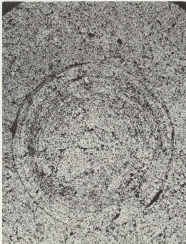
Figure 25. Hertzian Crack Produced by 0.29 J (Ballistic) on Impact Face of Dense SiC Unprotected by EAL
