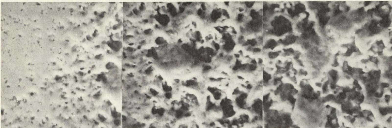
Figure 18. SEM Traverse from Dense Through Porous Zones with EAL Containing 1.0% Boron Sintering Aid (900X)
