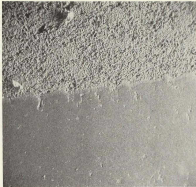
Figure 11. SEM at Interface of SiC Duplex Structure with EAL Containing 0.5% Boron Sintering Aid (20X)
