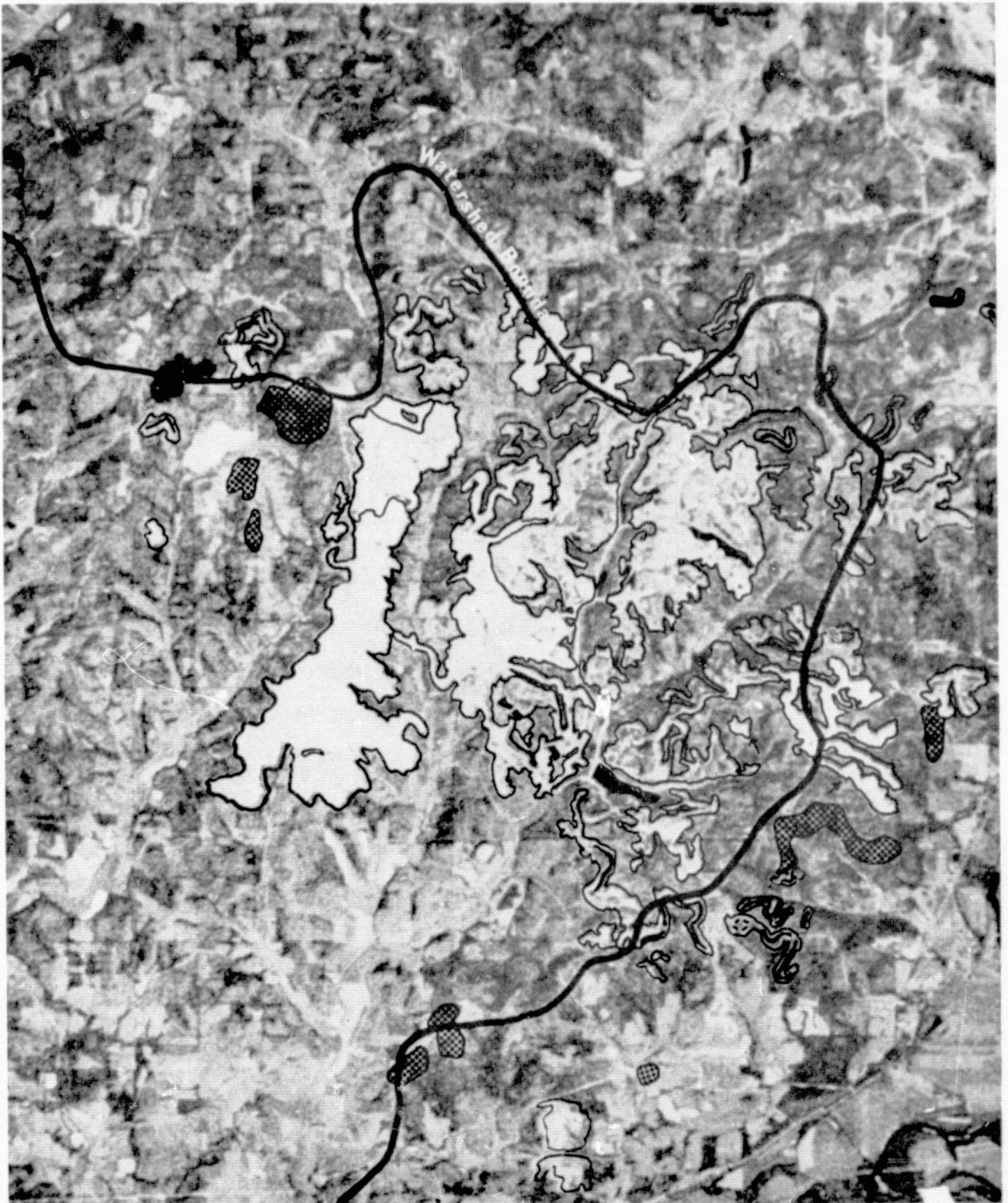
FIGURE 15. WATERSHED IN SOUTHEASTERN COSHOCTON COUNTY, OHIO WITH STRIP MINED LAND AS DELINEATED FROM SKYLAB S190B COLOR IR. Scale 1:80,000
