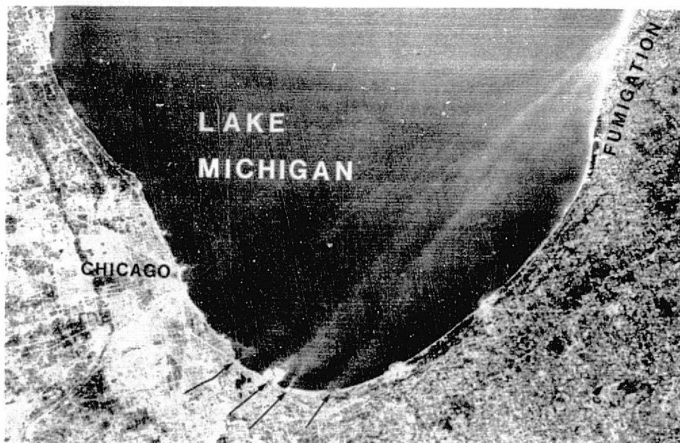
Figure 8. - Landsat-I, band 5, image of Chicago, Gary and southern Lake Michigan, 1003 LST, 14 October 1973. Smoke plumes advect across relatively cold lake showing little diffusion, only to fumigate on downwind shoreline near Benton Harbor, Michigan.
