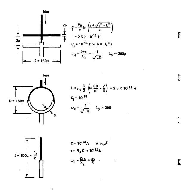
Figure 1.- Tank circuits resonating in the far infrared. Capacitance in the lumped circuits are dominated by the junction capacitance.
