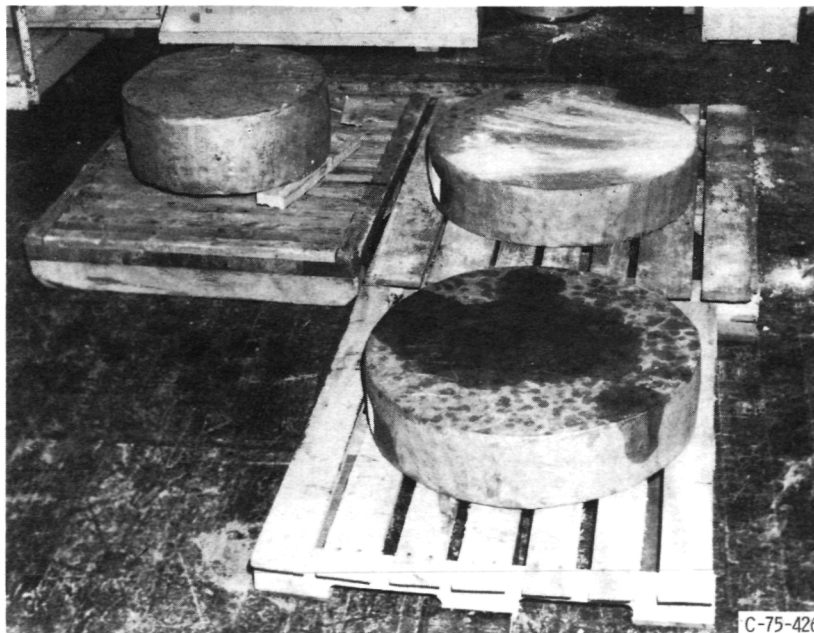
Figure 12. - Pitch change gear blank forgings.
