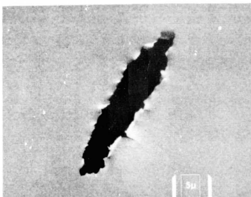
Figure 13. Elongated hole in gold foil
