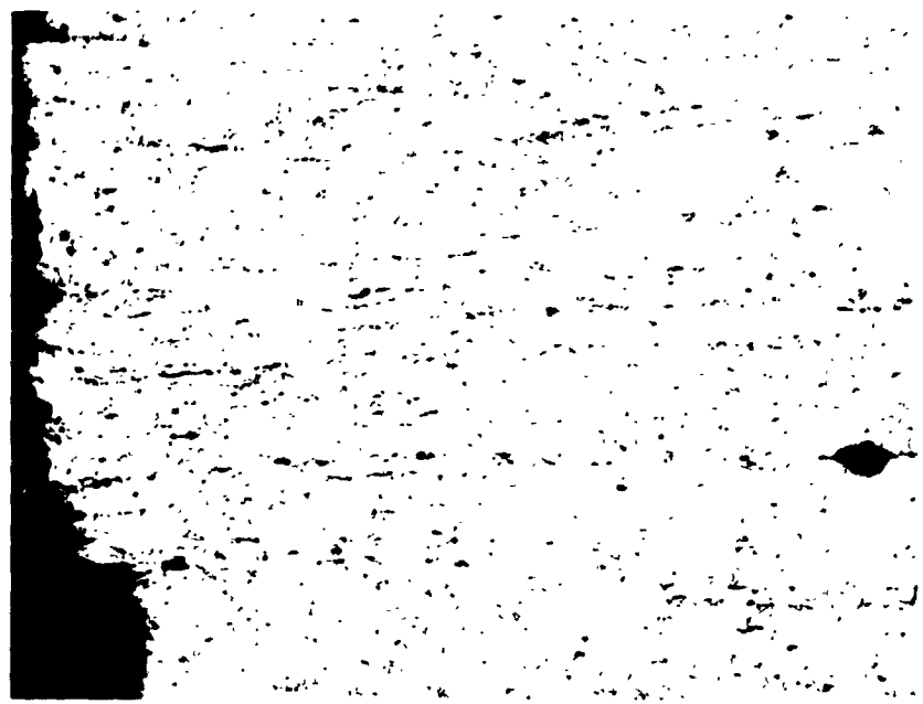
b. Longitudinal section through specimen about 6.35 mm (0.25 in.) from fracture.
