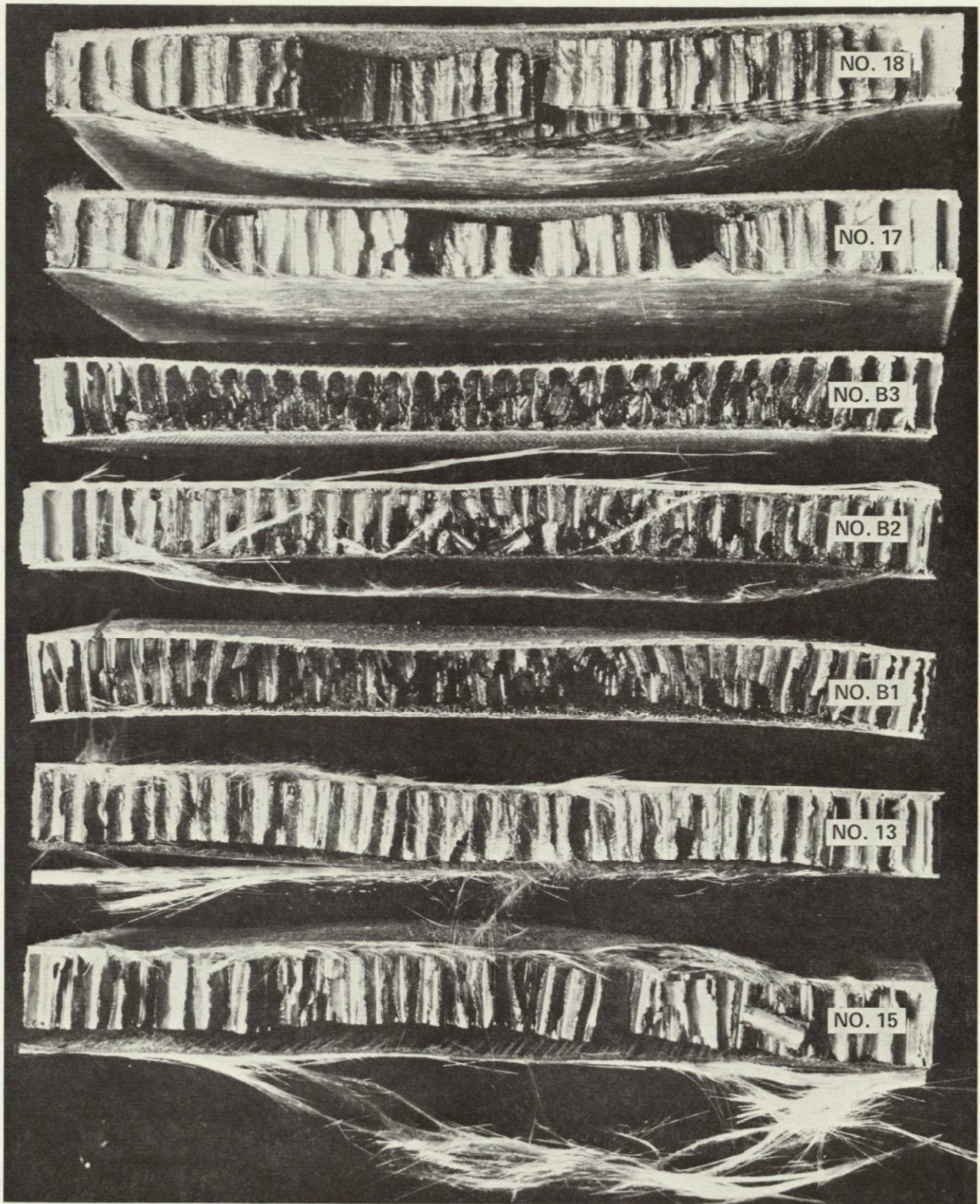
Figure 25.—Burn-Through Test Showing Typical Internal Damage—Section View of Test Specimens, 10-min Test
