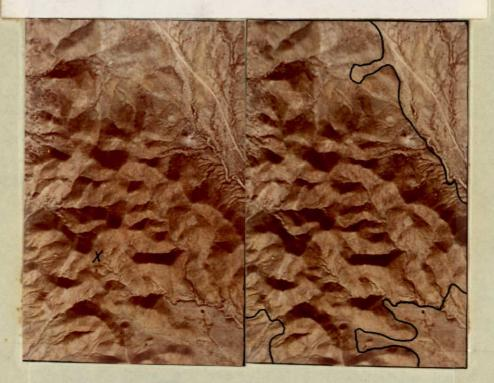
Each stereo pair was cut out and glued to 5" x 8" cards to facilitate ease of handling and stereo viewing. These were placed on the card in proper orientation to the flight line and spaced for stereo viewing by "naked-eye" or with a pocket stereoscope. An identification number was placed on the front of each card and keyed to show the identification of the subject vegetation in the stereo pair. Only the author had access to this key.
