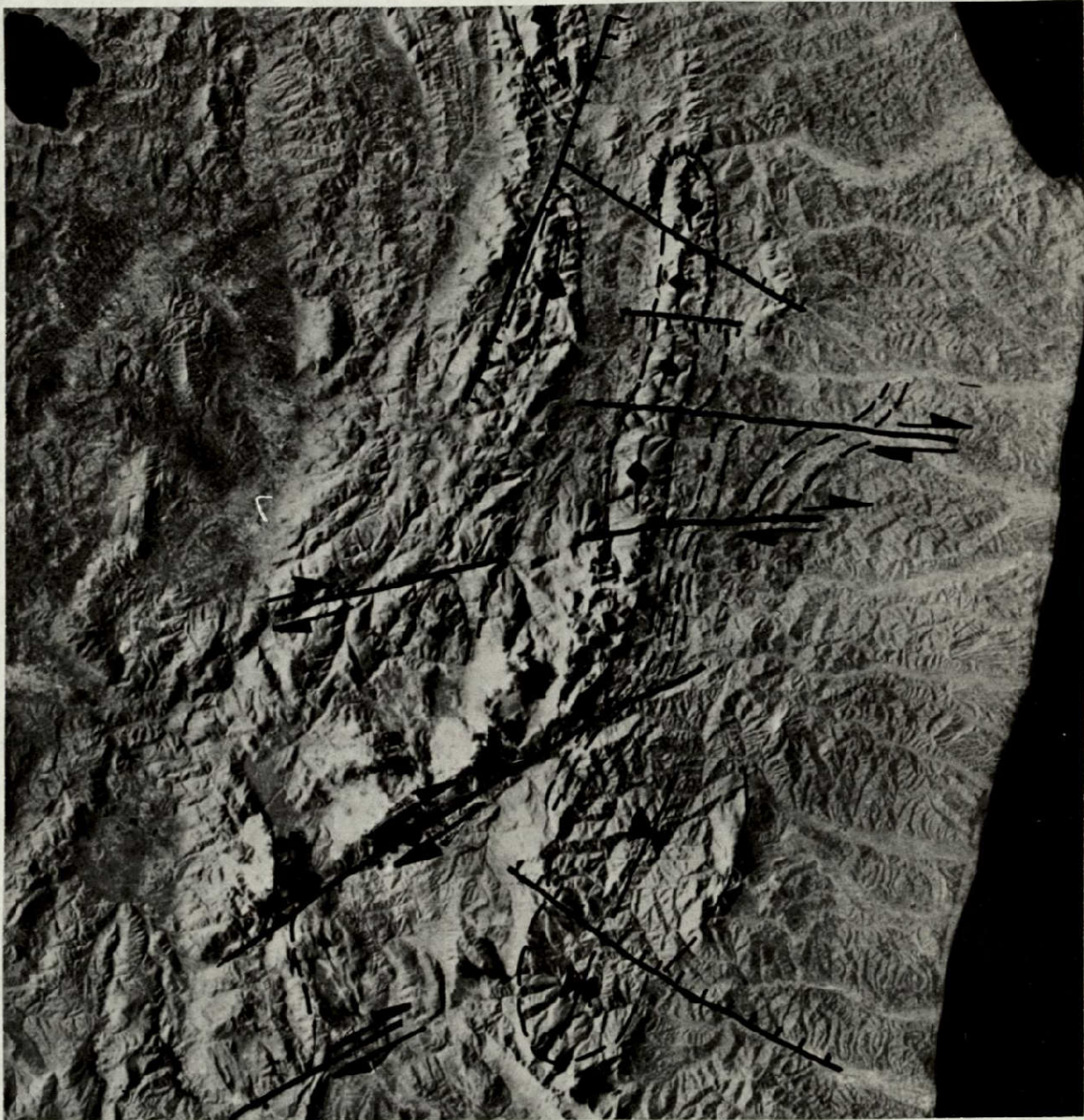
Fig. 4 Umbrian Arc, Skylab S 190 A; Examples for detecting faults by morphological features
