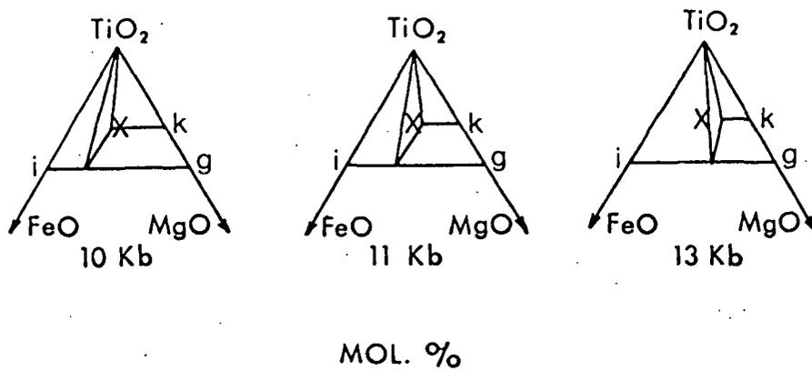
Fig. 2. Schematic illustration of the stages of isothermal (1200°C) decomposition of  $\text{MgFeTi}_4\text{O}_{10}$  with rising pressure. X = Fixed bulk composition ( $\text{MgO} \cdot \text{FeO} \cdot 4\text{TiO}_2$ ). i = ilmenite ( $\text{FeTiO}_3$ ); g = geikielite ( $\text{MgTiO}_3$ ), k = karrooite ( $\text{MgTi}_2\text{O}_5$ )
