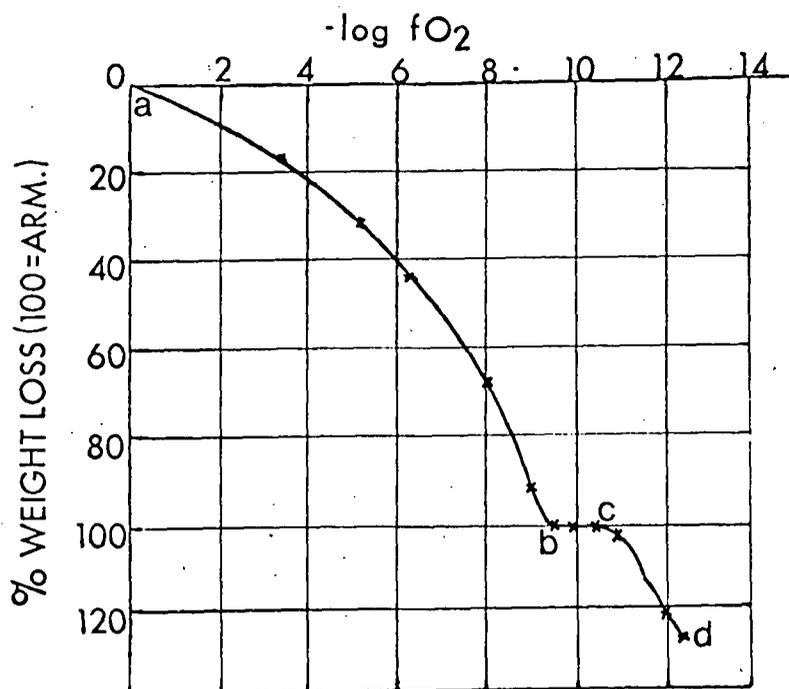
Fig. 4. Thermogravimetric stability curve for 1:1:4 (Mg:Fe:Ti) oxide compositions as a function of oxygen fugacity at 1200°C.
