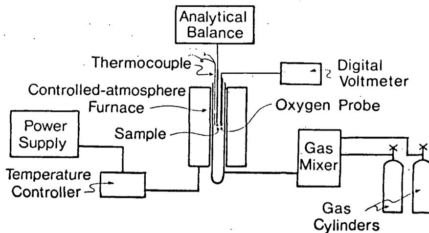
Fig. 1. Schematic diagram of system for thermogravimetry at controlled oxygen fugacities and at one atmosphere total pressure.
