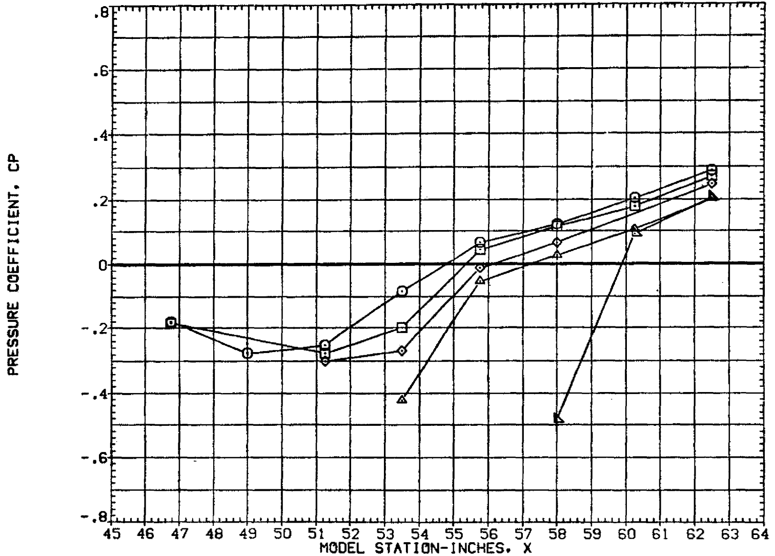
FIG 7 WING UPPER SURFACE STATIC PRESSURE DISTRIBUTION
