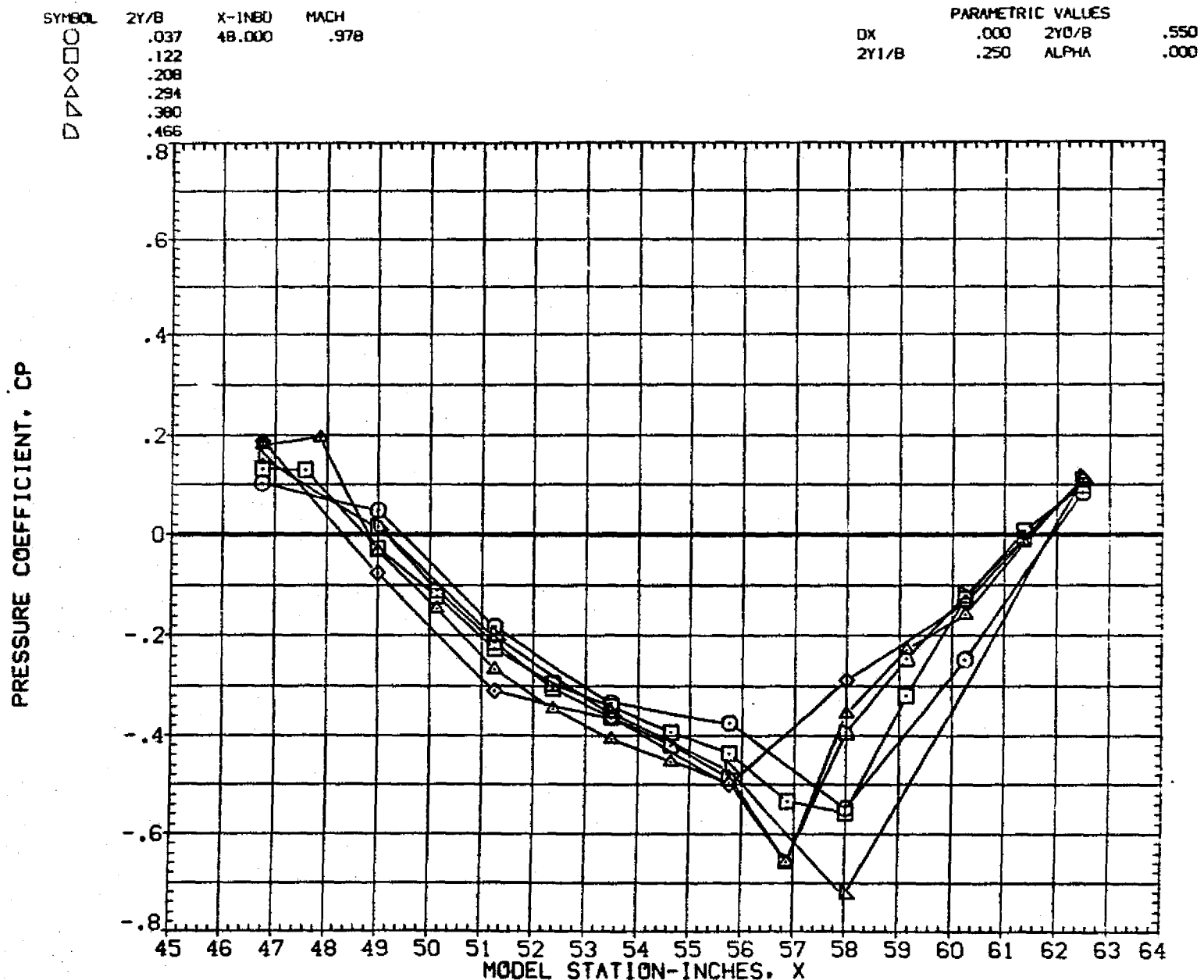
FIG 6 WING LOWER SURFACE STATIC PRESSURE DISTRIBUTION
