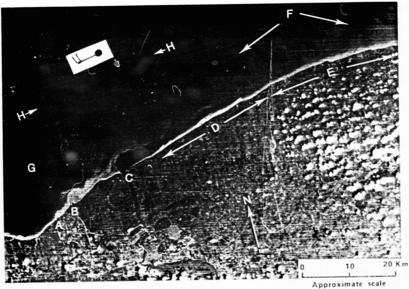
Figure 28. -- Part of LANDSAT-1 image 1280-15302, obtained April 29, 1973, showing Port Dalhousie (A), Welland Canal (B), Niagara River (C), beach erosion plumes (D and E), turbidity waves (F), offshore plumes (G and H).
