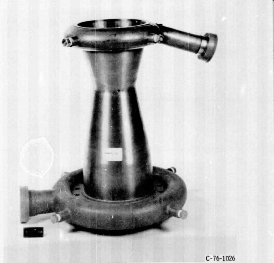
(f) COMPLETED FATIGUE CHAMBER (CONTOUR A). Figure 3. - Concluded.
