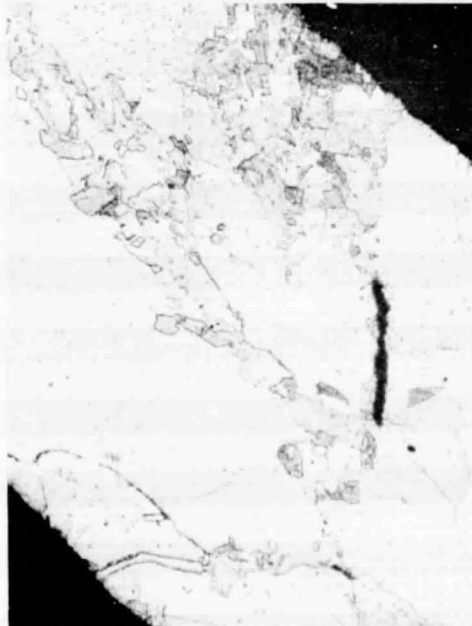
Figure 17. - Enlarged (X150) cross-sectional photograph showing recrystallization and cracking of grain boundaries with an OFHC copper chamber.
