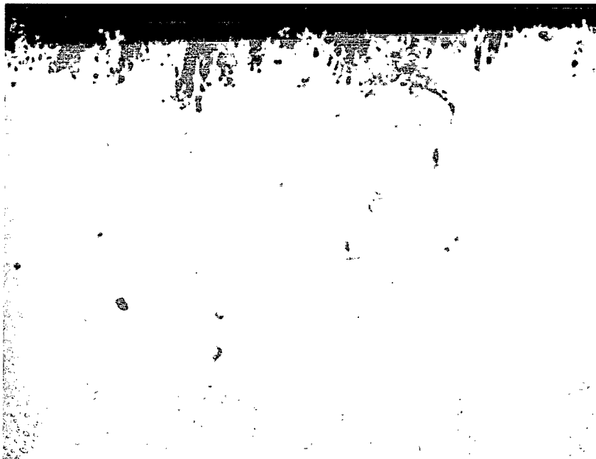
(b) 200 1-hour cycles at 1200° C. X100.
