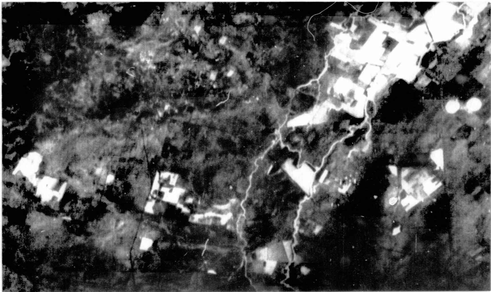
Fig. 16 - Survey of irrigated lands using the RB-57F, RS-7 scanner data. Area imaged is comparable to the photographic image in Fig. 1. The irrigated lands and surface water appear light in tone (cool). Approximate scale 1:100,000.
