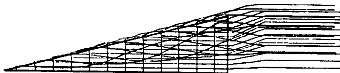
Figure 1.- A typical solution of the wake shape for a delta wing with R = 1 . 12 \times 12 lattice.
