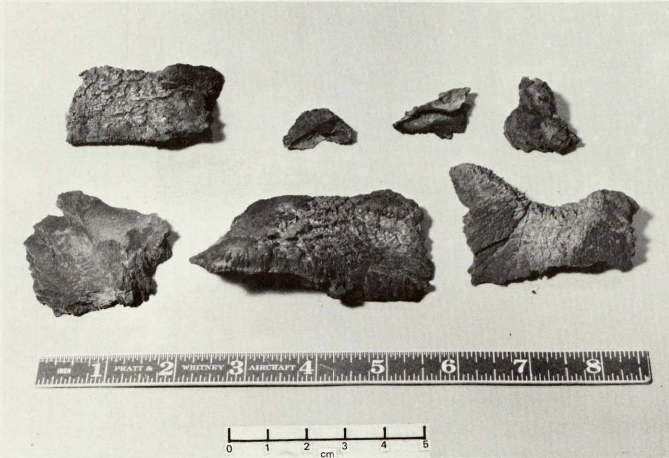
Figure 31 Carbon Deposits Removed from the Vorbix Combustor Pilot Zone Following the Four-Hour Idle Endurance Test on No. 2 Home Heat Fuel
