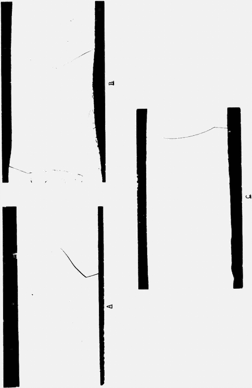
FIGURE 18: MICROGRAPHS OF SECTIONED PLATINUM COMPONENT OF A TEST THERMOCOUPLE AGED AT 1500°C AND AT A GRADIENT OF 1475°C/CM FOR 60 HOURS. WIRE DIAMETER WAS 0.51 MM; THE MAGNIFICATION WAS 90X. PHOTOGRAPH A SHOWS A SECTION TAKEN 1.0 CM FROM THE JUNCTION; B, 0.5 CM FROM THE JUNCTION; AND C, 0.05 CM FROM THE JUNCTION. FURTHER DESCRIPTION IS IN THE TEXT, 3.7.2. THERMO- COUPLE SYSTEM: PLATINUM-13% RHODIUM VERSUS PLATINUM.
