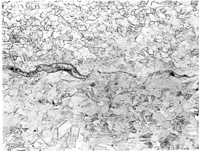
100X 10% Chromic Electro-Etch 1H866 a. Section CV-1A-1 (located near initiation end)
