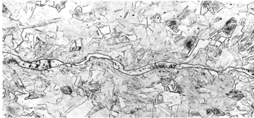
100X 10% Chromic Electro-Etch 1H868 a. Section CC-1-A (located near initiation end)
