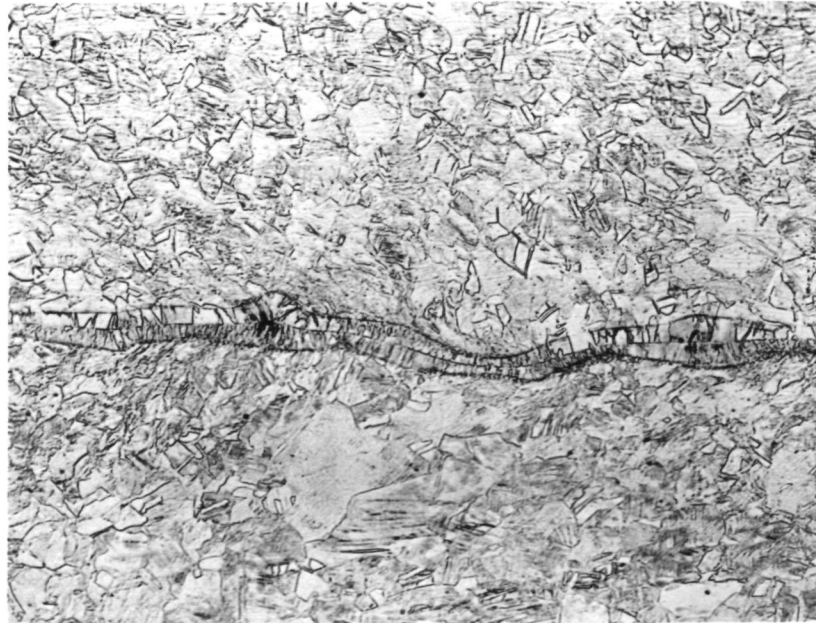
100X 10% Chromic Electro-Etch 1H867 b. Section CV-1A-2 (located in convex curvature)
