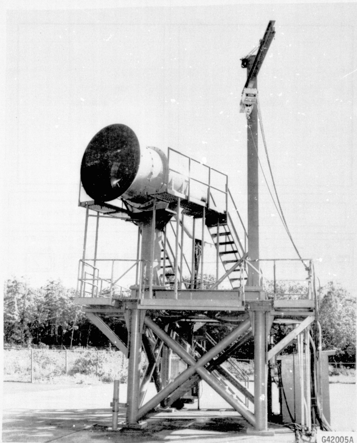
FIGURE 14. TEST RIG WITH Q-FAN INSTALLED - FRONT OBLIQUE VIEW
