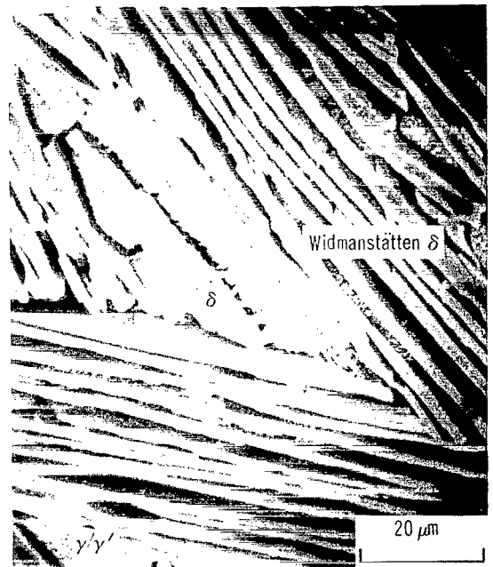
(b) SEM micrograph ( \gamma/\gamma' matrix etched out).
