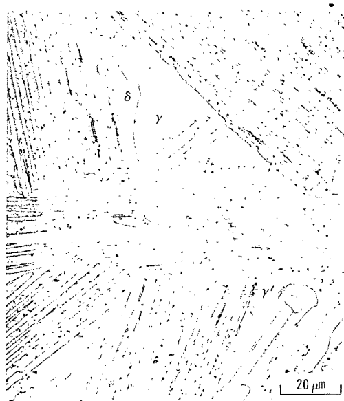
(a) Solution treatment, 4 hours at 1210° C, air quenched.
