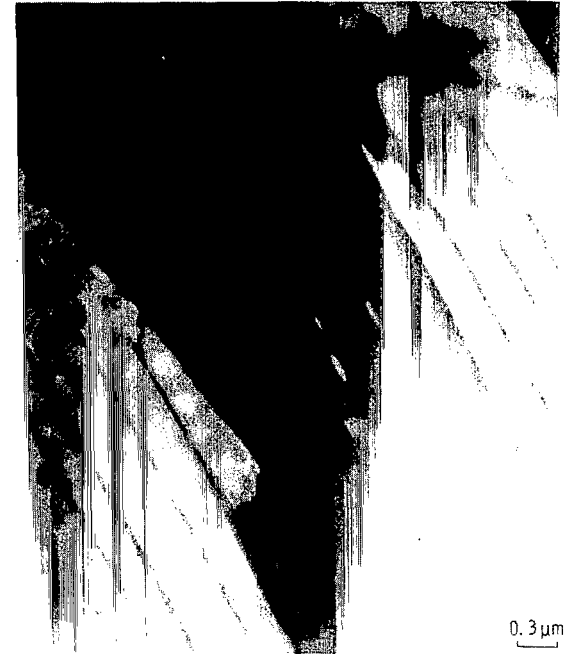
(c) Dark field electron micrograph showing fine precipitates in \delta region (see (a)) using 00\bar{2} \gamma diffraction point shown in (b).
