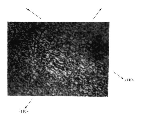
Fig. 3.8 Interference phase contrast photomicrograph of the surface of an APD structure. These surface features are between 1 and 2 fringes which corresponds to a height of 2700 to 5400Å.
