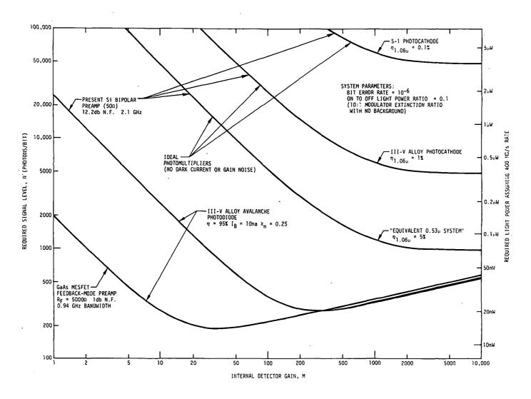
Fig. 2.3 Comparison of the calculated Performance of Various 1.06 $\mu$  Detectors as 400 Mb/s PGBM Modelocked Laser Communications Receivers. Plotted is the number of photons per bit required for  $10^{-6}$  bit error rate data reception as a function of internal detector gain.  $N_0$  = 175 electrons assumed for lowest curve GAASFET preamp as a goal; best performance achieved to date is  $N_0$  = 347 electrons for preamp #8, the curve for which would lie a factor of 2 above this for low M.
