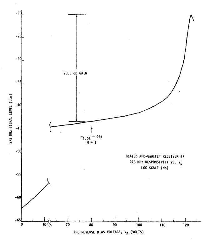
Fig. 4.6 High-Frequency Avalanche Gain versus APD Reverse Bias for the 5 mil diameter K-9 GaAs<sub>1-x</sub>Sb<sub>x</sub> APD in GAASFET Preamp #7 (a). Complete curve, including noise, for the final delivered GAASFET preamp #7 is shown in Fig. 4.21.
