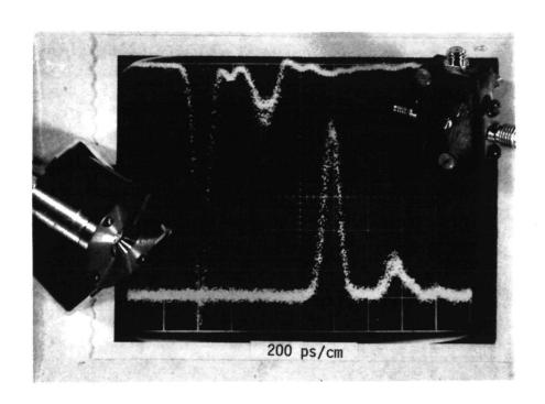
Fig. 4.3 Response of Two 3 mil M8-l Inverted Heterojunction Microwave Avalanche Photodiodes to Modelocked Nd-YAG Laser Pulses. Upper curve (inverted) is from older mount (Ref. 1) shown on left into S-4 sampler, whereas lower (upward-going) curve is for similar APD in the new compact 50Ω mount shown at the upper right and Fig. 3.ll into an S-6 sampler. Both curves at 200pS/cm. Note the clean fall and return to baseline between the two laser pulses for the new diode mount.
