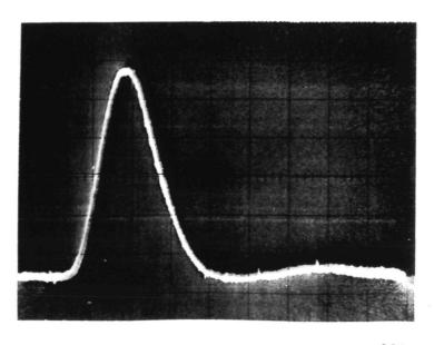
c) 500pS/cm showing response to isolated "l". This would be the same as the current impulse response if the modelocked laser pulsewidth were short enough.
