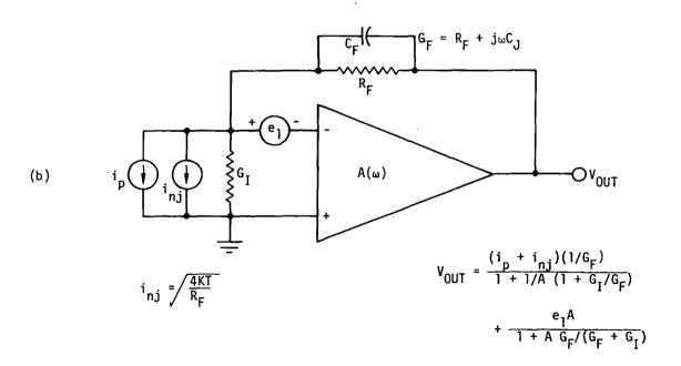
Fig. 2.8 Signal and Noise Models for Feedback-Mode (Transimpedance-Type) Preamps. a) General case of feedback element with (Frequency-dependent) noise voltage
