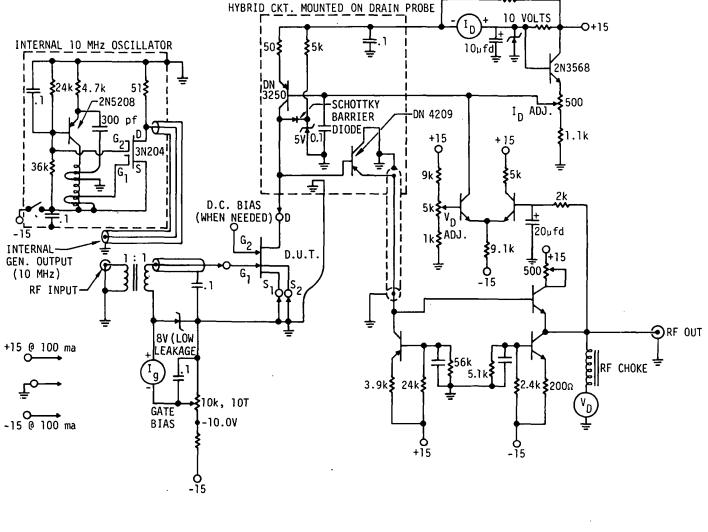
Fig. 3.13 Circuit Diagram For Active Probe Test Setup for Measuring Open-Circuit Gain of GAASFET's. The hybrid 1C chip, 0.200" square, is mounted near the end of the probe so that the drain is supplied from a high impedance, low capacitance current source.
