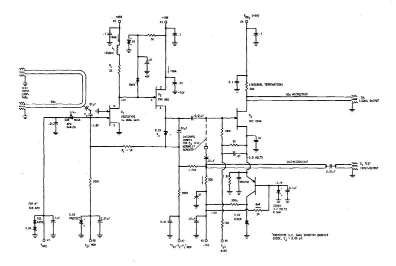
Fig. 4.24 Circuit Diagram of the Mark III GAASFET Preamp Design with specific values for Preamp #8.
