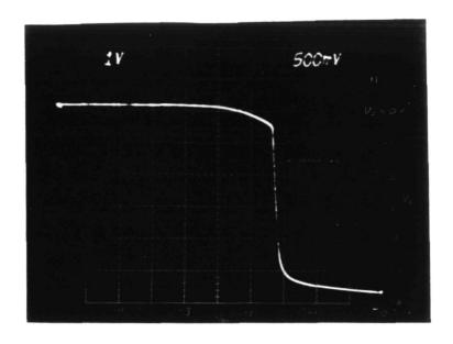
Fig. 4.30 Open-Loop dc Transfer characteristic of the  $Q_1-Q_2$  "op-amp" in Preamp #8. Horizontal is  $V_{g1}$  (1 V/cm, zero at right) and vertical is  $V_F$ , the op-amp dc output voltage (0.5V/cm, zero 2 cm from top). Normal feedback operation point is at  $V_F = V_{D1} = -1.65V$ .  $V_{DS}$  of  $Q_1 \simeq V_F + 6.2$  volts.
