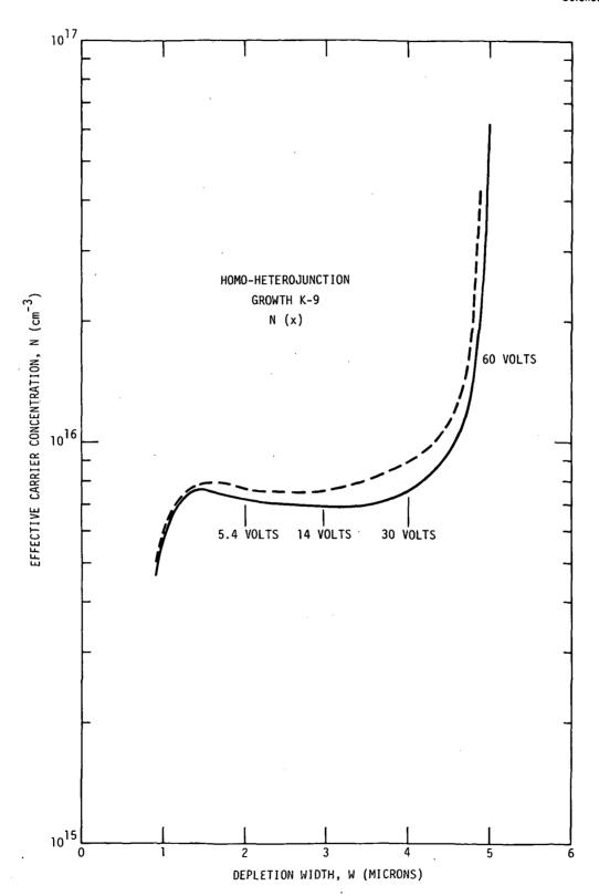
Fig. 4.1 Carrier Concentration versus Depth, N(X), measured on two different 5 mil diameter diodes on the K-9 epitaxial growth used for these homo-heterojunction APD's (structure of Fig. 2.7).
