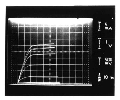
Fig. 4.27 I<sub>D</sub> vs. V<sub>DS</sub> curves for GaAs MESFETS in Preamp #8.
