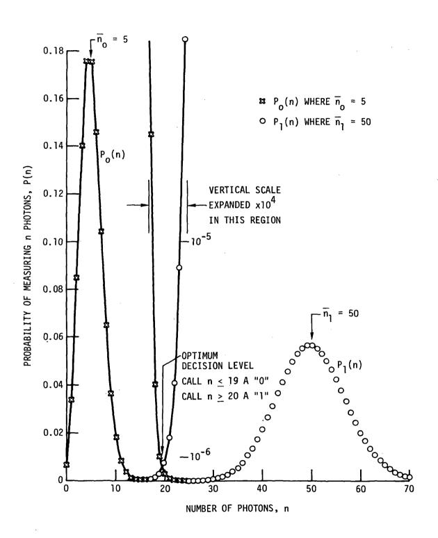
Fig. 2.1 Example of Optical Detection in the Poisson (counting statistics) Limit. For  $\overline{n}_1 = 50$ ,  $\overline{n}_0 = 5$ , optimum decision level is to call n>20 a "1" and n<19 a "0", for which we obtain an average probability of error per bit of BER =  $4.12 \times 10^{-7}$ .
