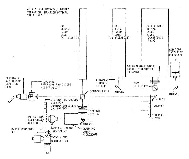
Fig. 3.14 Diagram of the optical table layout used for this work, including the 1.06 $\mu$ m (modelocked), 1.152 $\mu$ m, and 6328Å lasers and the scanning light microscope.
