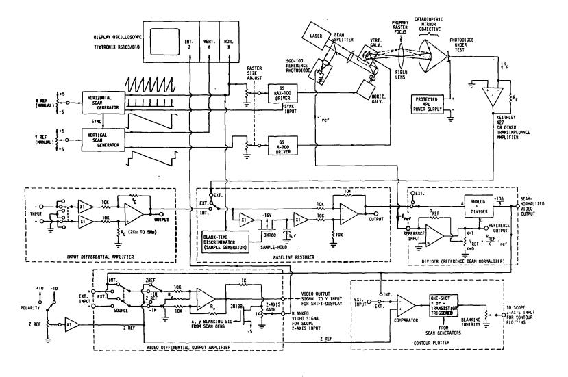
Fig. 3.15 Block-Diagram of the Scanning Laser Microscope System.
