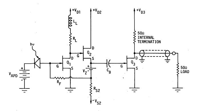
Fig. 2.12 Simplified Circuit Diagram of the Mark III GAASFET Preamp Design. (Complete circuit diagram for GAASFET preamp #8 is shown in Fig. 4.24.)
