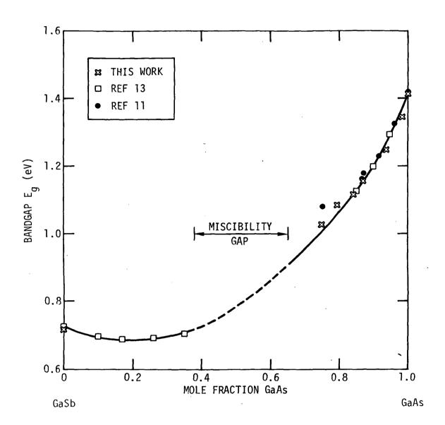
Fig. 3.4 Energy bandgap vs. composition for the GaAs(1-x)Sb<sub>x</sub> alloy system. The region 0.4<x<0.65 is inaccessible because of a miscibility gap in the alloy.
