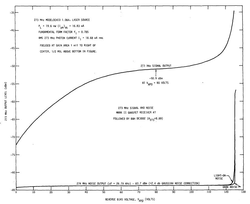
Fig. 4.21 Variation of 273 MHz Signal Output and Illuminated and Dark Noise Outputs for Mark II GAASFET Preamp #7 (b) with final delivered APD.
