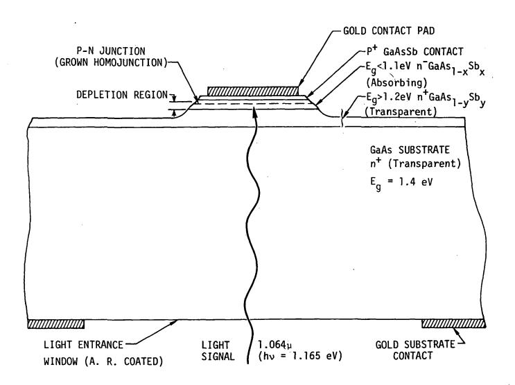
Fig. 2.7 Device Structure for an Inverted Homo-Heterojunction GaAs<sub>1-X</sub>Sb<sub>X</sub> Avalanche Photodiode. Note that as opposed to the earlier structure of Fig. 2.5, the peak electric field is at a p-n homojunction produced during continuous growth of the n<sup>-</sup> active (absorbing) layer by adding a small amount of p-type dopant to the melt. The device is normally operated with the n<sup>-</sup> layer completely depleted.
