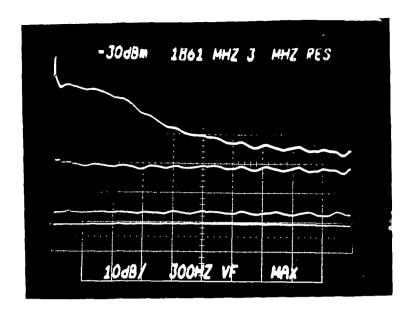
Fig. 4.20 Noise output spectra from Mark III GAASFET Preamp #7.
