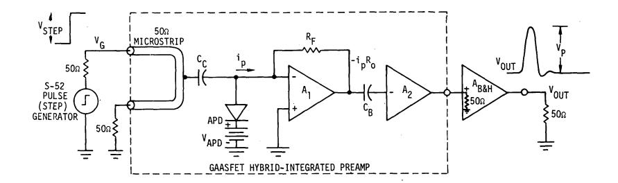
$$Q_{p} = i_{p}dt = C_{C} V_{STEP}$$
