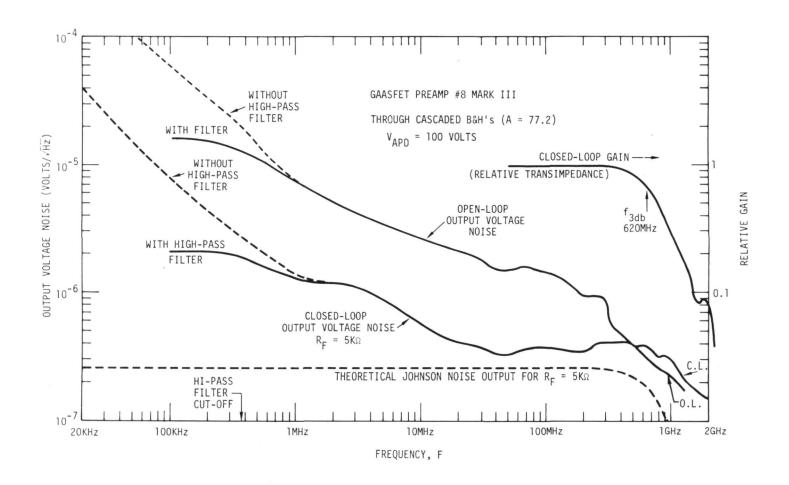
Fig. 4.38 Spectral Dependence of Noise Output Voltage (Open-Loop and Closed-Loop) for Mark III GAASFET Preamp #8.
