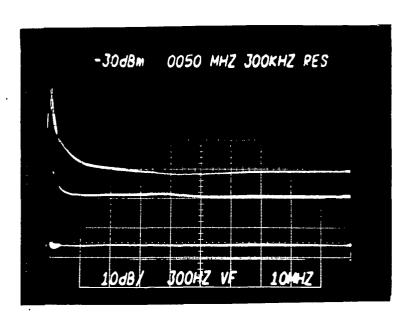
b) 0 to 100 MHz Frequency Range (10 MHz/cm). The thermal noise for  $R_F=3K\Omega$  would be -72.4dBm.
