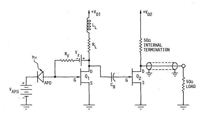
Fig. 2.9 Simplified Circuit Diagram for the Mark IA GAASFET Preamps Design. (Complete circuit diagram is shown in Fig. 4.9.)
