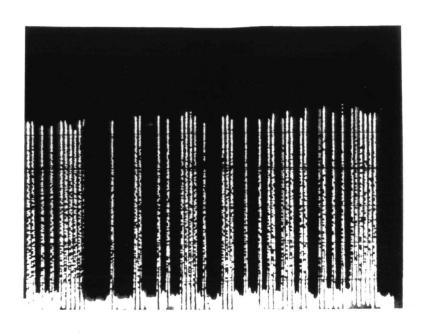
Fig. 4.39 Response of GAASFET Preamp #8 with 5 mil APD to 400 Mb/s  $1.06\mu$  PGBM modelocked laser data stream. Measured on McDonnell-Doublas Test Communications System. 10mV/cm vert. (through B&H DC 3002 preamp). ( $I_p$ )AVE= $1\mu$ A.
