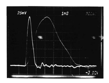
Fig. 4.35 Current impulse response of Mark III GAASFET Preamp #8 (signal-averaged result from Fig. 4.34) displayed at 25mV/cm vertical, lns/cm and (light trace) 200ps/cm horizontal.
