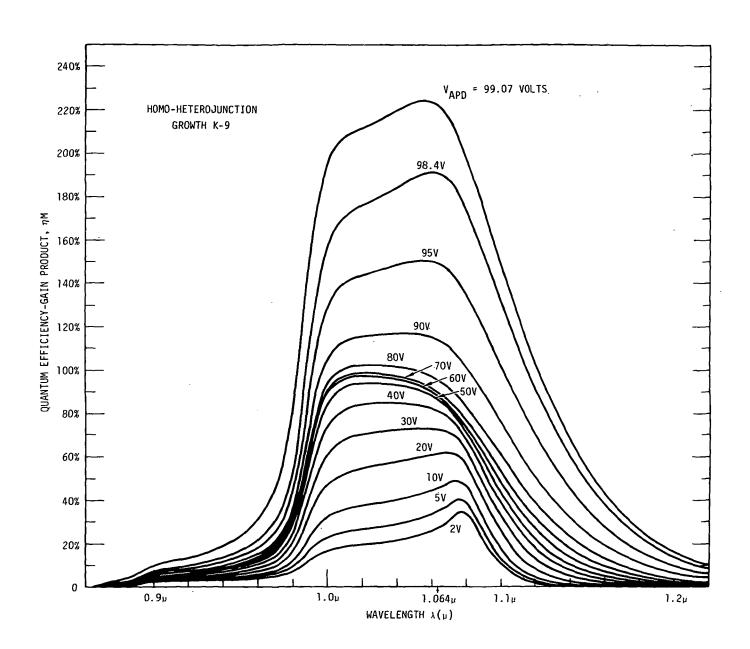
Fig. 4.5 Spectral Photoresponse for a 5 mil Diameter K-9 APD for Biases from VAPD = 2 volts to VAPD = 99.07 volts. Ordinate is quantum efficiency (quantum efficiency-gain product for VAPD>70 volts) versus wavelength. More typical K-9 APD's as used in the GAASFET receivers have 15% to 20% higher VB's and  $0.01\mu$  to  $0.02\mu$  longer wavelength response than this particular device.
