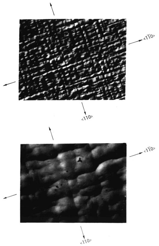
Fig. 3.7 Normarski phase contrast photomicrographs of the surface details of an APD structure. Note the alignment of surface features along <110> directions.
