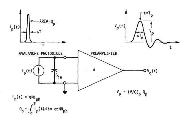
Fig. 2.2 Schematic of Avalanche Photodiode Receiver Defining Response Parameters.
