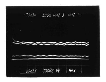
Fig. 4.29 Noise Output Spectra from the output stage Preamp #8 with the gate of Q3 termiminated  $25\Omega$  to ground. Measured through cascaded B&H preamps.
