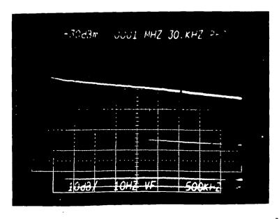
c) 0 to 5 mMz Frequency Range (500 KHz/cm). No high-pass filter used. The thermal noise for  $R_F=3K\Omega$  would be -80.0dBm.
