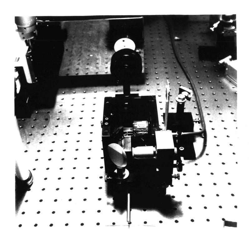
Fig. 3.16 a) Photograph of the Scanner Unit of the Scanning Laser Microscope taken along the direction of the exit beam. Beam enters the GCO401 spatial filter from the right.
