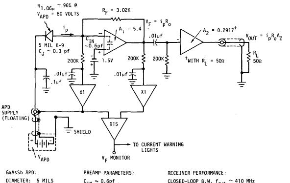
Gaassb APD: PREAMP PARAMETERS: RECE DIAMETER: 5 MILS  $C_{IN} \approx 0.6 pf$ . CLOS  $C_{J} \approx 0.3 pf$  OPEN-LOOP GAIN  $A_{I} = 5.4$  PULS  $\eta_{1.06u} \approx 96\%$  ( $V_{APD} \geq 80V$ )  $(f_{3db} = 32.5 \text{ MHz})$  THRO  $V_{B} = 116.5V$  OPEN-LOOP GAIN-BW  $\sim 1.2 \text{ GHz}$  PEAK GAIN  $M_{MAX} \approx 8$   $A_{2} = 0.2917 \text{ INTO } 50\Omega \text{ LOAD}$   $R_{F} = 3.02 K\Omega$   $R_{O} \approx \frac{R_{F}}{1+(1/A_{I})} = 2548\Omega$
