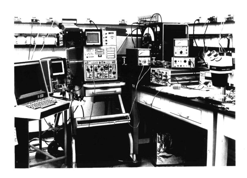
Fig. 3.20 Measurement Equipment Routinely Used For GAASFET Preamp Evaluation, including the Tektronix Digital Processing Oscilloscope.
