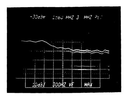
Fig. 4.15 Noise output spectra from GAASFET Preamp #4 through cascaded B&H's.
