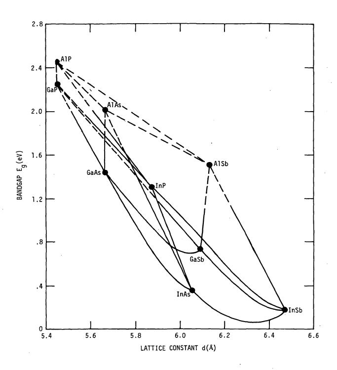
Fig. 3.1 Energy bandgap vs. lattice constant for all of the binary and ternary alloy semiconductors of Al, Ga or In with P, As or Sb. The solid lines are for direct bandgap materials and the dashed lines for indirect bandgap materials.
