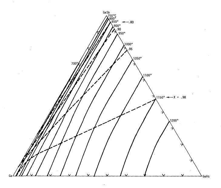
Fig. 3.2 Ga rich region of the GaAsSb phase diagram. The solid lines are liquidus isotherms while the dashed lines are  $GaAs_XSb(1-x)$  isocomposition lines.
