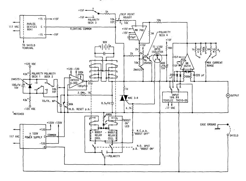
Fig. 3.18 Circuit Diagram for the Precision  $\pm$  200 volt Floating APD Supply.
