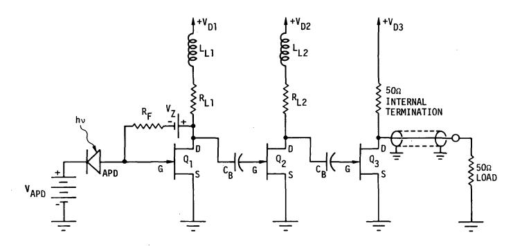
Fig. 2.11 Simplified Circuit Diagram for the Mark II GAASFET Preamp Design. (Complete circuit diagram for preamp #7 is shown in Fig. 4.16.)
