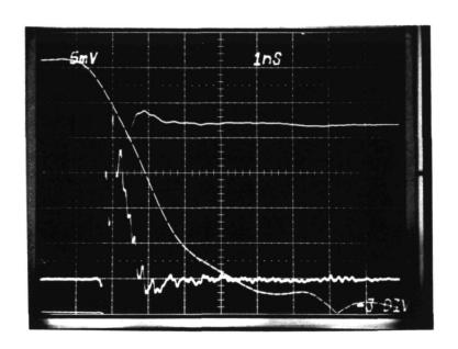
Fig. 4.36 Current impulse response of GAASFET Preamp #8 with  $V_{APD}$  = 100V measured directly into S-6 (without B&H preamps). Input Step;  $V_{STEP}$ =0.2442 volts through internal  $C_{C}$ . Current impulse at 5mV/cm, 1 ns/cm, zero 3 cm below center. Integral at 2pVs/cm, lns, zero at bottom (-4cm). FFT at 150 $\mu$ V/cm, 256 MHz/cm horizontal, with f=0 at left edge (vertical zero at bottom).
