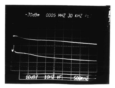
c) 0 to 5 MHz Frequency Range (500 KHz/cm). The thermal noise for  $R_F=5K\Omega$  would be -77.24 dBm. Noise output measured through OSM 201103A blocking capacitor (375 KHz hi-pass filter).
