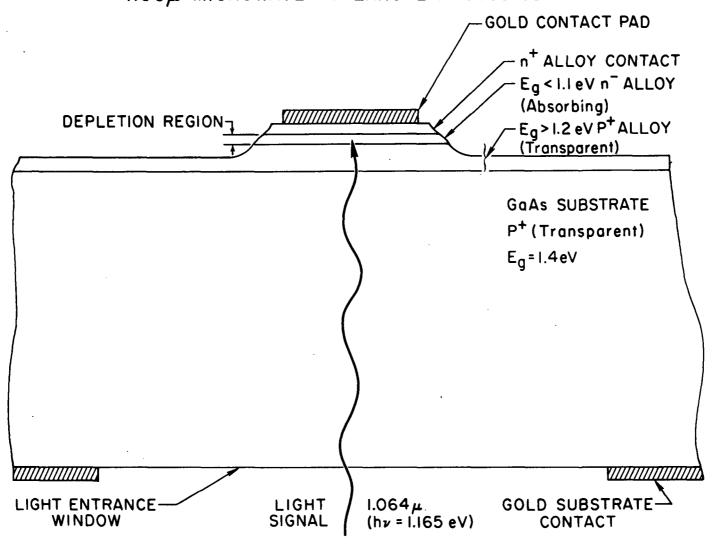
Fig. 2.5 Original Inverted Heterojunction III-V Alloy Microwave Avalanche Photodiode Design. Note that the peak electric field (high avalanche gain) region is at the p<sup>+</sup> (transparent buffer layer) - n<sup>-</sup> (absorbing active layer) heterojunction interface.
