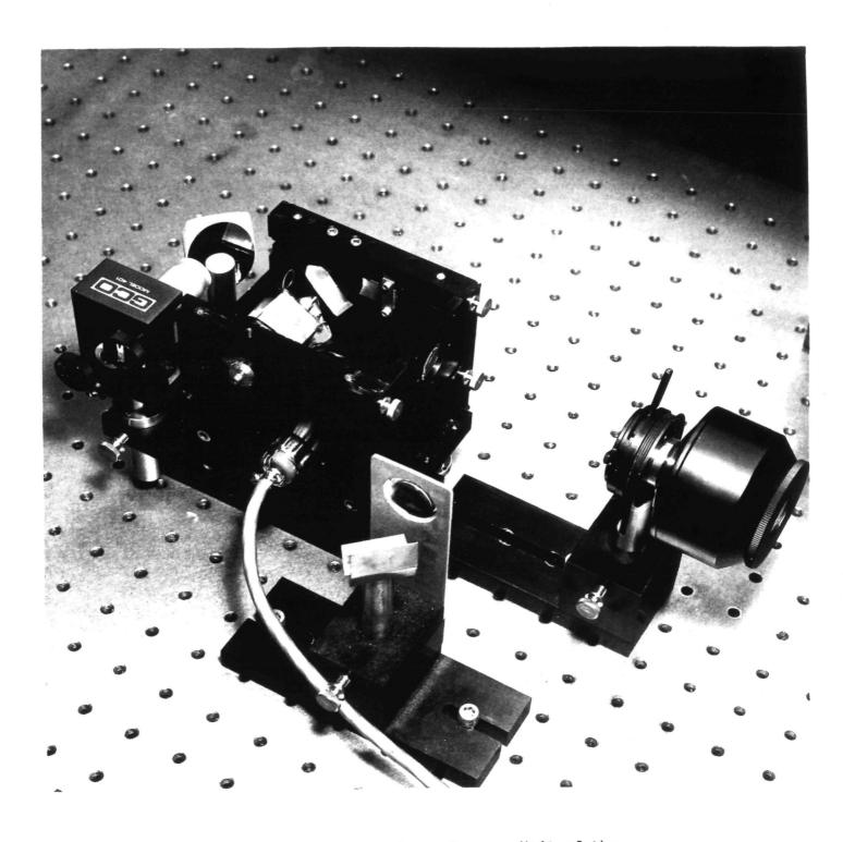
Fig. 3.16 b) Another view of the Scanner Unit of the Scanning Laser Microscope with the 40X 0.5NA Catadioptric Mirror Objective at the right.
