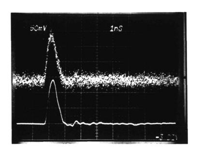
Fig. 4.34 Current impulse response of GAASFET Preamp #8 (with  $V_{APD}$  = 100 volts) to a 4125-electron current impulse (receiver output amplified thru cascaded B&H wideband  $50\Omega$  amplifiers). Upper curve output directly as seen on sampling oscilloscope (12.15 mV rms voltage noise). Lower curve is a 1024 waveform signal average of output. Both curves at 50 mV/cm, 1 ns/cm.
