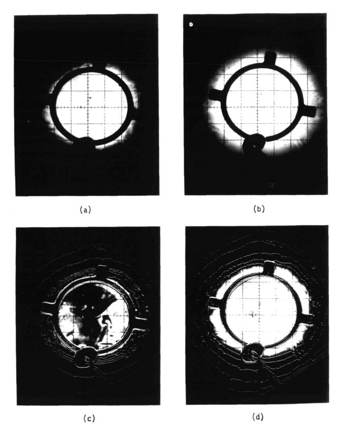
Fig. 3.17 Scanning light microscope micrographs of response of a Si photodiode at 6328Å. (a) and (b) intensity modulated display for diode at 0 and 20 volts bias respectively. The dark ring indicating no response is the Ohmic contact to the diode. (c) and (d) are a combined intensity modulation and contour mapping display of the same diode at 0 and 20 volts bias respectively.
