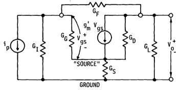
b) Reduced AC Equivalent Circuit, where
