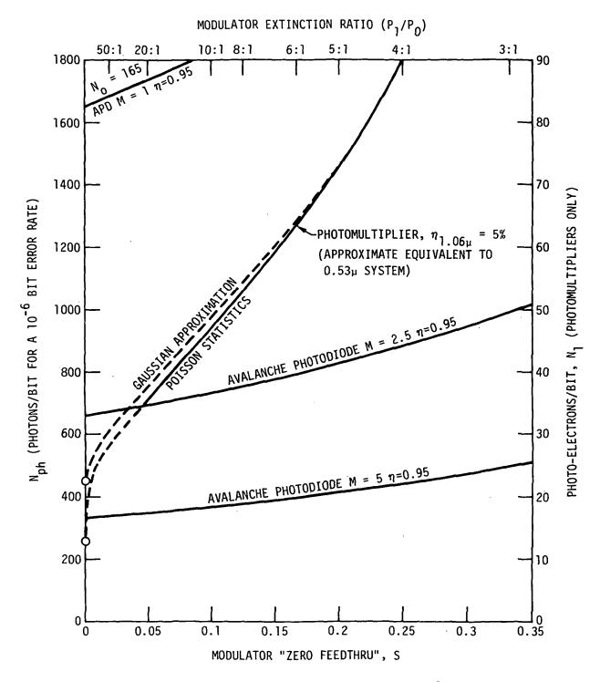
Fig. 2.4 Calculated Signal Level to Achieve a 10<sup>-6</sup> B.E.R. Versus Modulator Zero Feedthrough or Extinction Ratio for Photomultipliers (or Other Poisson Statistics Receivers as Compated to a Preamp-Noise-Limited Receiver (APD Receiver at Low M).
