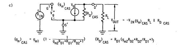
Fig. 2.13 Circuit Model For Cascode FET Arrangement Illustrating the Greatly Increased Voltage Gain of a Dual-Gate GAASFET Compared to a Single-Gate. a) Cascode equivalent circuit for a dual gate GAASFET. b) Low-frequency (omitting capacitances) model for a). c) Equivalent circuit for b) defining the equivalent drain resistance and equivalent transconductance for the dual-gate FET or cascode arrangement. Note that (RD)CAS>>RD.
