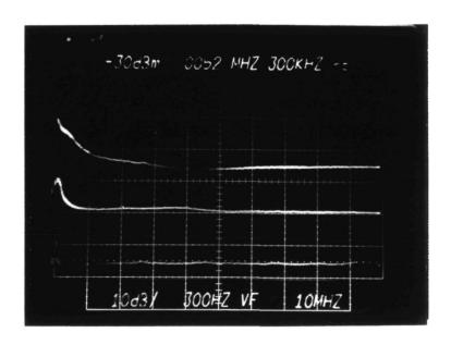
b) 0 to 100 MHz Frequency Range (10 MHz/cm). The thermal noise for RF= $5K\Omega$  would be -68.38 dBm.
