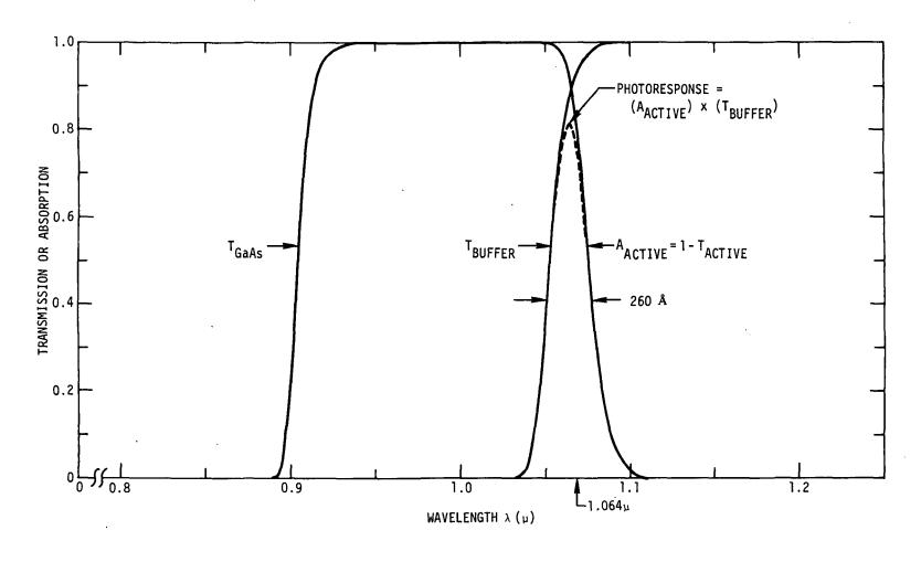
Fig. 2.6 Example of Spectral Photoresponse Which Can Be Obtained in Either Inverted Heterojunction or (Fully Depleted) Inverted Homo-Heterojunction Avalanche Photodiode. While this illustrates narrowband photoresponse which can be obtained, usual experimental devices are made with wider response peaks and near 100% quantum efficiencies.
