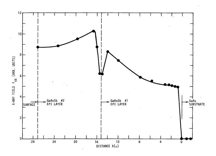
Fig. 3.5 Sb profile obtained from X-ray emission on SEM for two GaAsSb layers grown on a GaAs substrate. The melt composition for each epitaxial layer was identical but growth conditions at the time the second melt was brought over the substrate caused the Sb concentration to dip at the interface.
