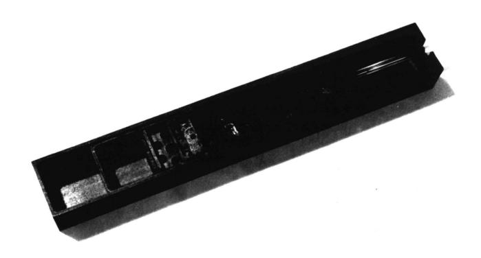
Fig. 3.6 Graphite slider boat used for "doping drop" growths. Top slider (small insert with holes) is where the dopant is placed and the quartz push rod is used to push this slider back to where the sets of holes line up and the dopant drops through into the melt to change the doping.
