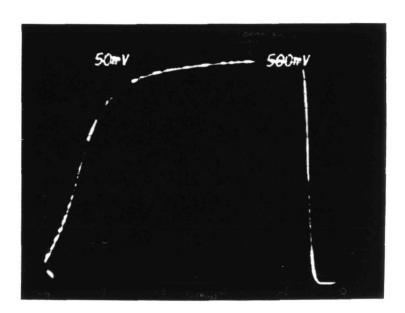
Fig. 4.31 100 MHz Open-Loop Gain of Mark III GAASFET Preamp #8. Vertical is linear display of 100 MHz output, -30 dBm full scale, Horizontal is V<sub>F</sub>, 0.5 volts/cm (zero at right). Measured gain at balance is  $A_{12}$   $A_{3}$  = 17.5 dB.
