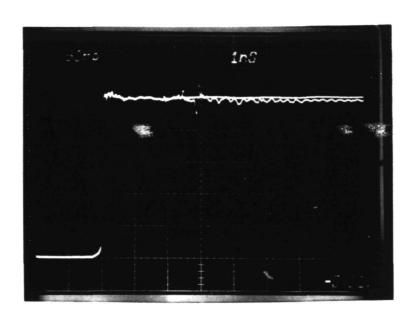
Fig. 4.28 Output time domain reflectometry traces for GAASFET Preamp #8 and a precision  $50\Omega$  reference termination (upper trace is right). 50mV/cm vertical, lnS horizontal, 30 ps time resolution.
