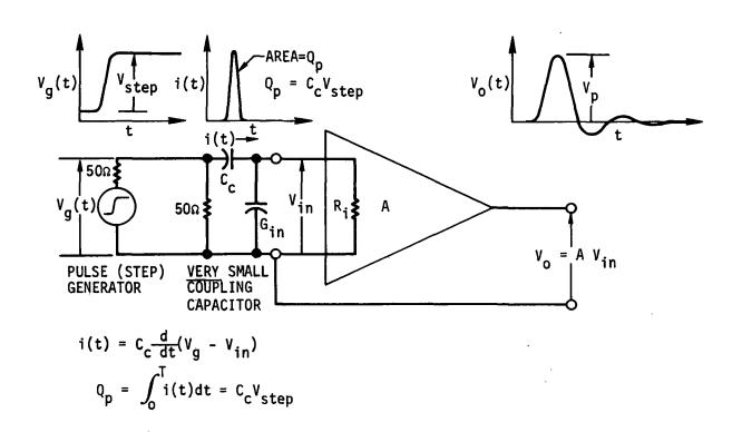
Fig. 3.22 Measurement Approach for Determining Current Pulse Response and  $(v_p/Q_p)$  for a Preamplifier.
