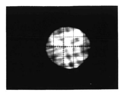
Fig. 4.22 Scanning light microscope pictures of the 273 MHz photoresponse of Mark II GAASFET Preamp #7. Scale is 1 mil/div.
