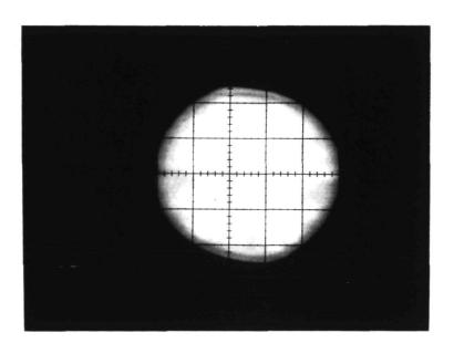
b) V<sub>APD</sub> = 110 volts Normal Contrast Intensity Modulation
