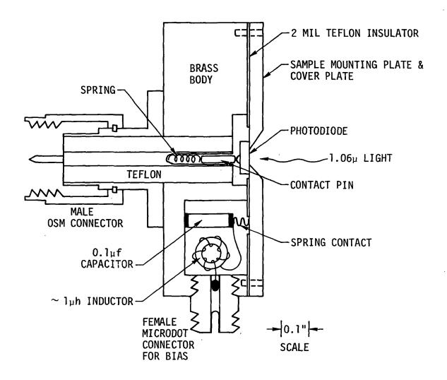
Fig. 3.11 New Compact 50Ω Microwave Mount for Inverted Heterojunction Microwave Avalanche Photodiodes. Internal LC filter attenuates RFI on APD bias power supply. Note that the front sample mounting and cover plate floats at the APD substrate bias, so exposed metal should be covered with a suitable insulation if danger of accidental contact exists. Fig. 4.3 shows a photograph of this mount with an APD pulse response.
