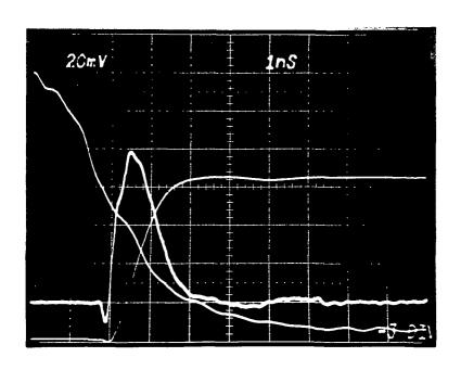
Fig. 4.14 Current Impulse Response for Mark IA GAASFET Preamp #4 Measured Through Cascaded B&H's. Input pulse was  $N_e$  = 8005 electrons. Current impulse response displayed at 20 mV/cm vertical (zero 3 div below center), lnS/cm horizontal, with integral at 20 pVS/cm. Also shown is the FFT-derived frequency response, displayed at 250 $\mu$ V/cm vertical (zero at bottom), 204.8 MHz/cm horizontal (zero at left edge).
