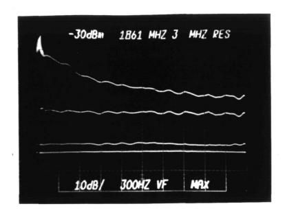
Fig. 4.33 Open-Loop Noise Output Spectrum from GAASFET Pream #8. Q1 in balance,  $V_F = -1.65 \text{ Vdc}$ , gate of Q1 terminated  $25\Omega$  to ground. Measured through cascaded B&H preamps.
