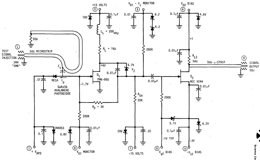
Fig. 4.9 Circuit Diagram for Mark IA Preamp Design with specific values for GAASFET Preamp #5.
