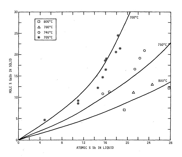
Fig. 3.3. Experimental and calculated Sb distribution curves for GaAsSb solid.
