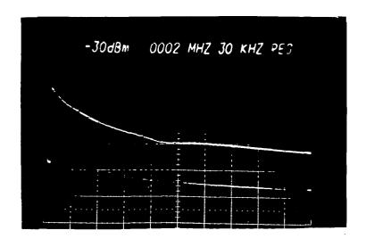
c) 0 to 5 MHz Frequency Range (500 KHz/cm). The thermal noise for  $R_F=3K\Omega$  would be -81.3dBm.
