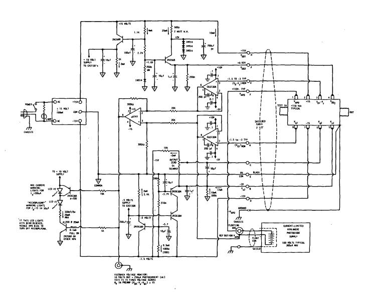
Fig. 4.10 Circuit Diagram for the Power Supply-Monitor Unit for the Mark IA GAASFET Preamps (#4 and #5). Note that Power Supply units are not interchangeable between preamps.
