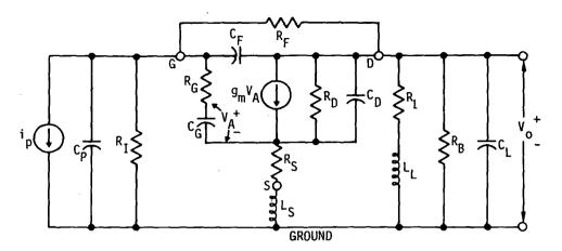
a) AC Equivalent Circuit for 3-NODE Analysis.
