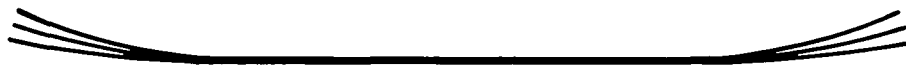
Figure 2-3. (b) Diagram of a Line Image From a Single Reflection Showing the End Spreading Due to the Synclastic Bending.
