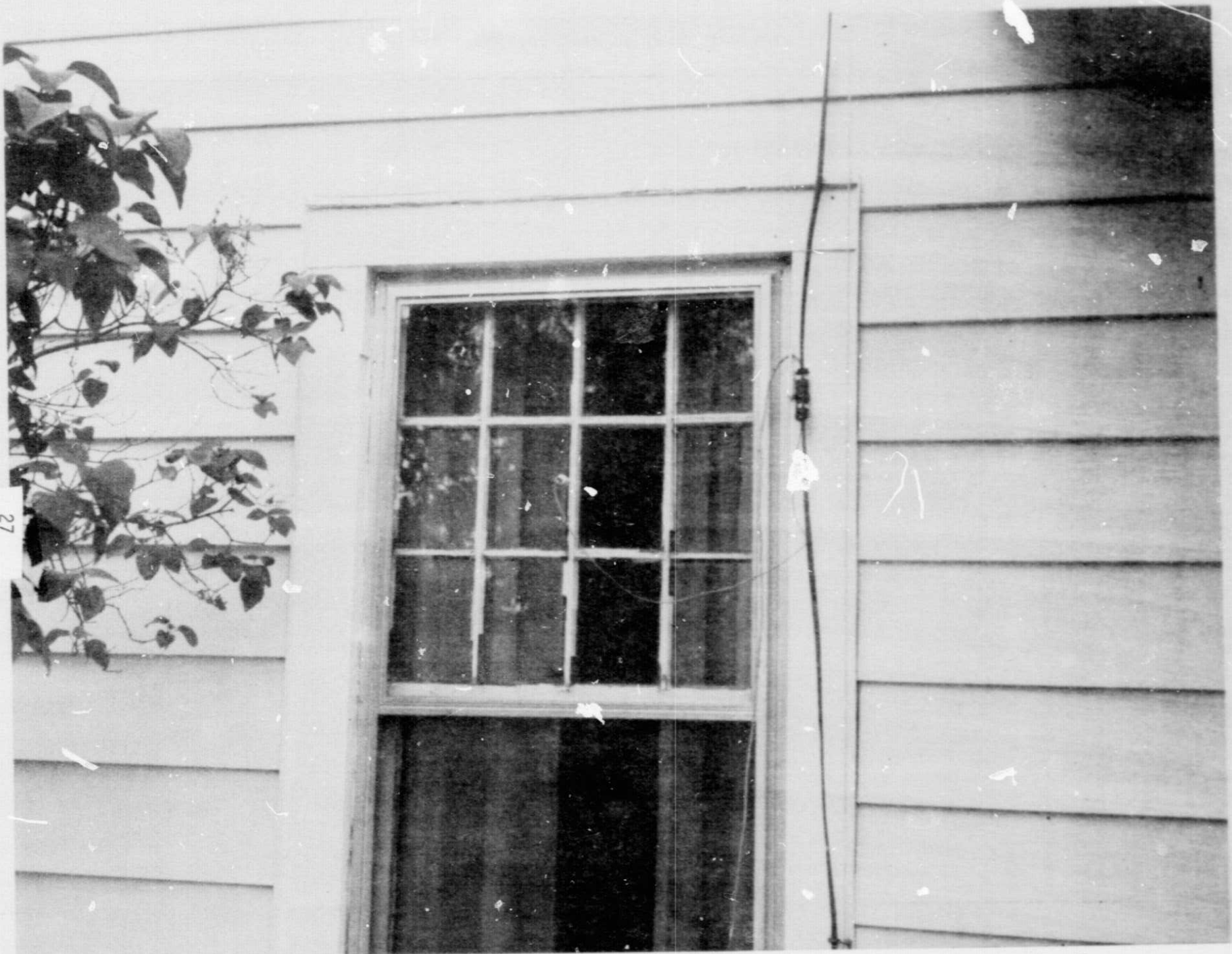
Figure 2(d). Location of accelerometer for window vibration measurements. Site 2.
