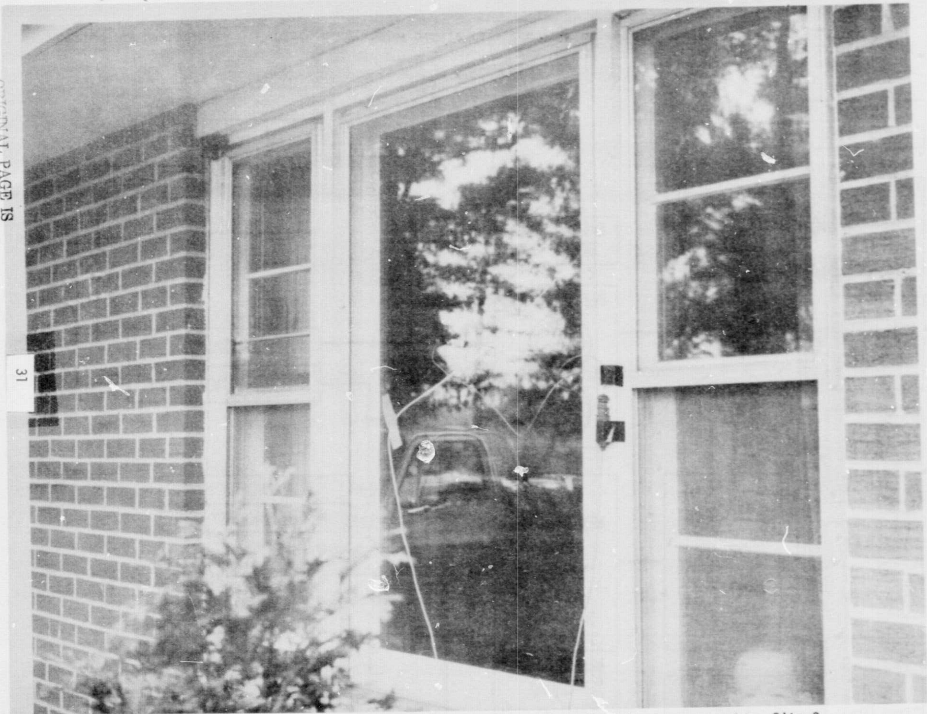
Figure 3(d). Location of accelerometer for window vibration measurements. Site 3.
