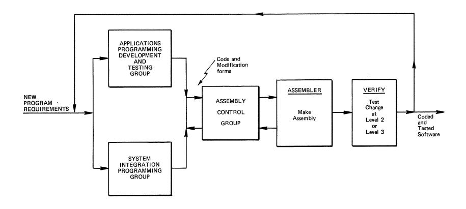
Fig. 4. Program & Assembly Control Activity
