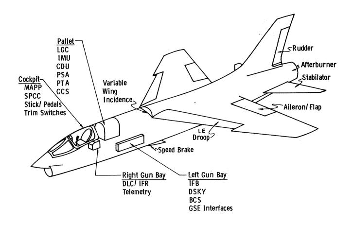
Fig. 1. F-8C DFBW Aircraft and Hardware
