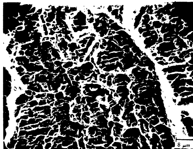
Fig. 17. SEM photomicrograph of rapid fracture in air by intergranular ductile rupture along low-angle subgrain boundaries of unaged weld (MJS-W-1)
