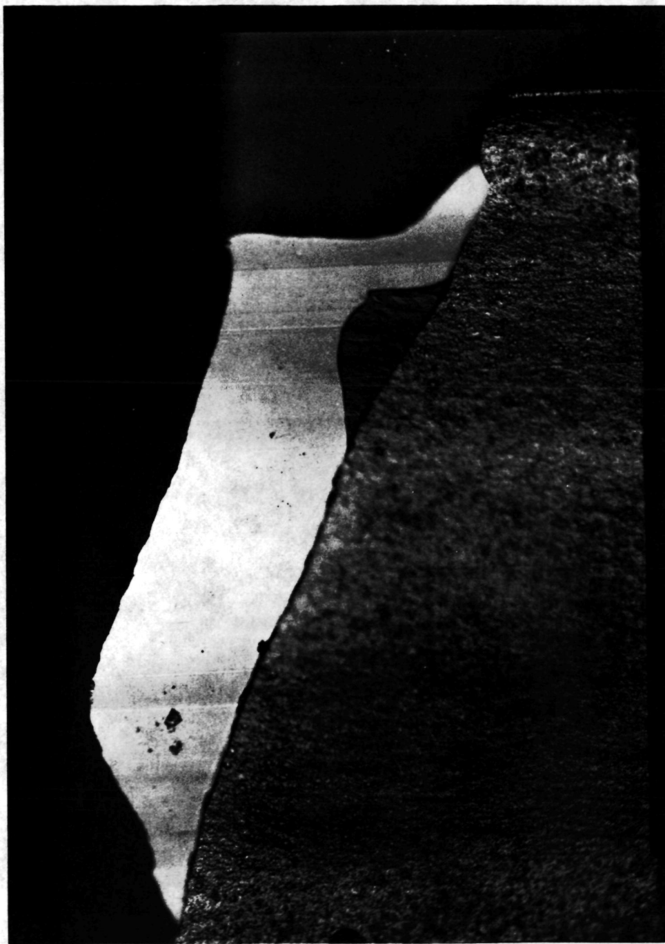
Figure 7 SIDE VIEW OF THE BROKEN END OF A SiC RIBBON
