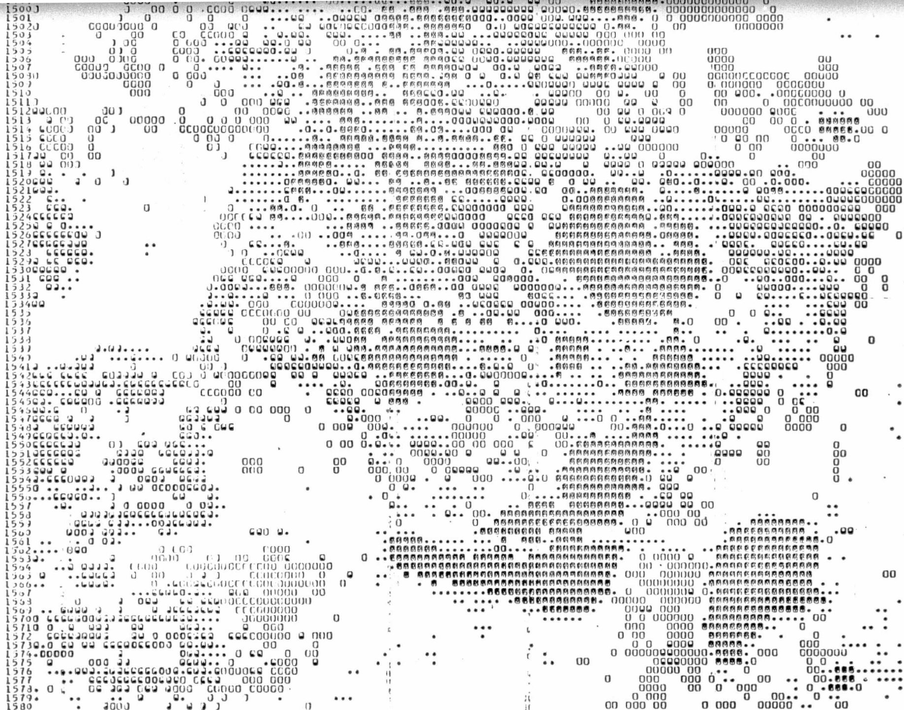
FIG.14. - Map from an early version of INTERPRET Multiple print was used to obtain a gray level presentation for the dif- ferent classes.
