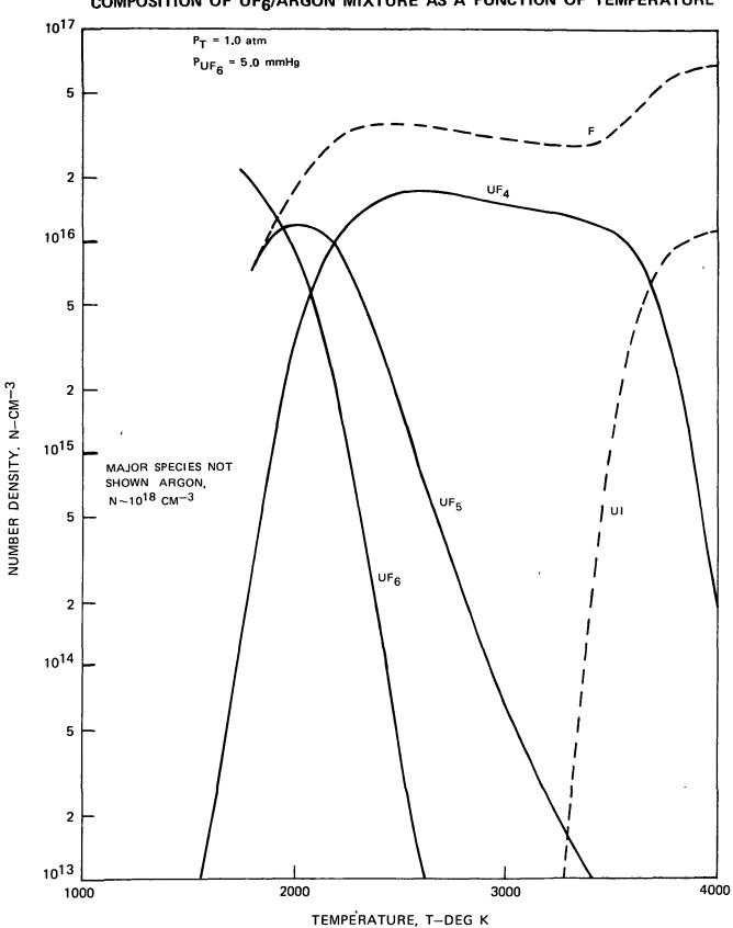
COMPOSITION OF UF6/ARGON MIXTURE AS A FUNCTION OF TEMPERATURE
