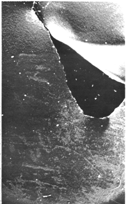
c) FAILED PORTION OF BURST DISC
