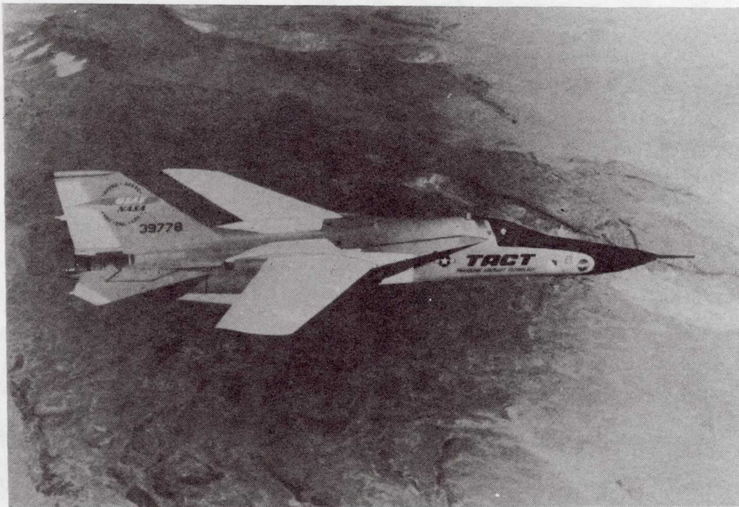
Figure 8.- U.S. Air Force F-111 with supercritical wing (TACT).
