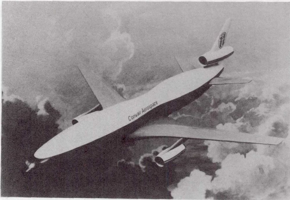
Figure 13.- Artist's concept of a near-sonic transport incorporating a supercritical wing.
