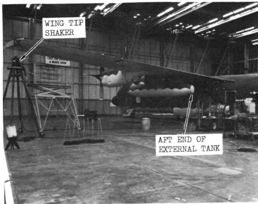
FIGURE 32. - GROUND VIBRATION TEST SETUP (OVERALL VIEW)
