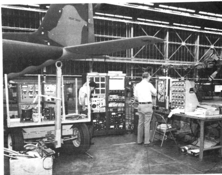
FIGURE 34. - GROUND VIBRATION TEST - DETAIL OF CONTROL AND RECORDING EQUIPMENT
