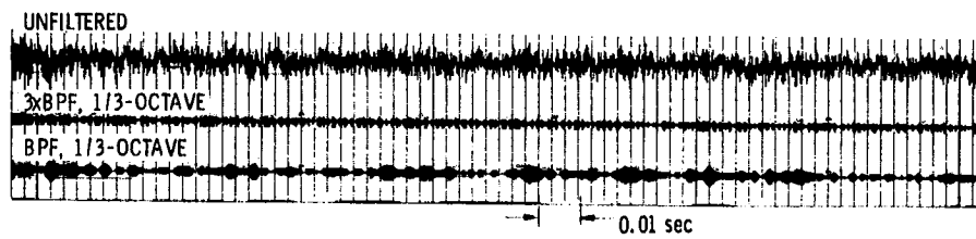
Figure 10. - Comparison of fluctuations in BPF tone level with those of its third harmonic (3x BPF); microphone is at 40°, and fan is at 3800 rpm.
