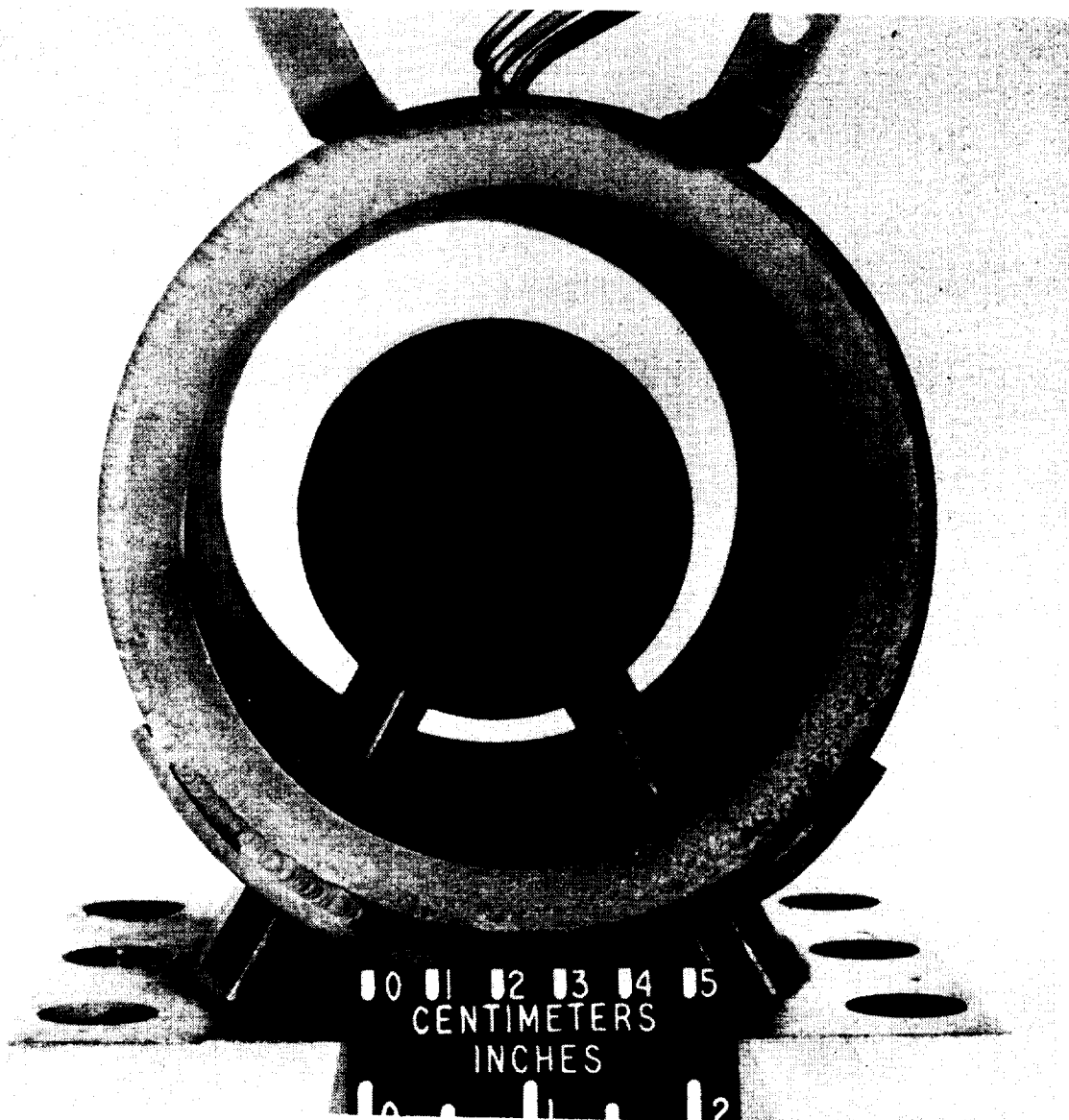
Figure 23.- Forward view of the HRE model with shroud, simulated instrumentation-cooling-water discharge system, and adverse-pressure-gradient barrier.
