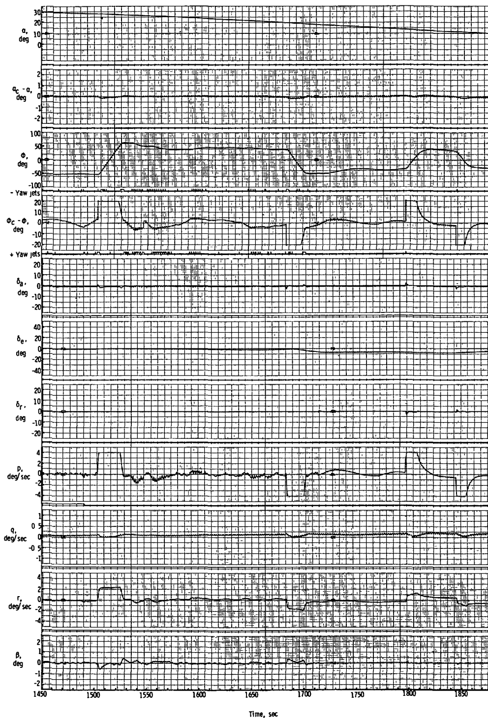
Figure 6.- Simulation strip charts for later portion of entry with guidance sampling time of 2.00 sec.
