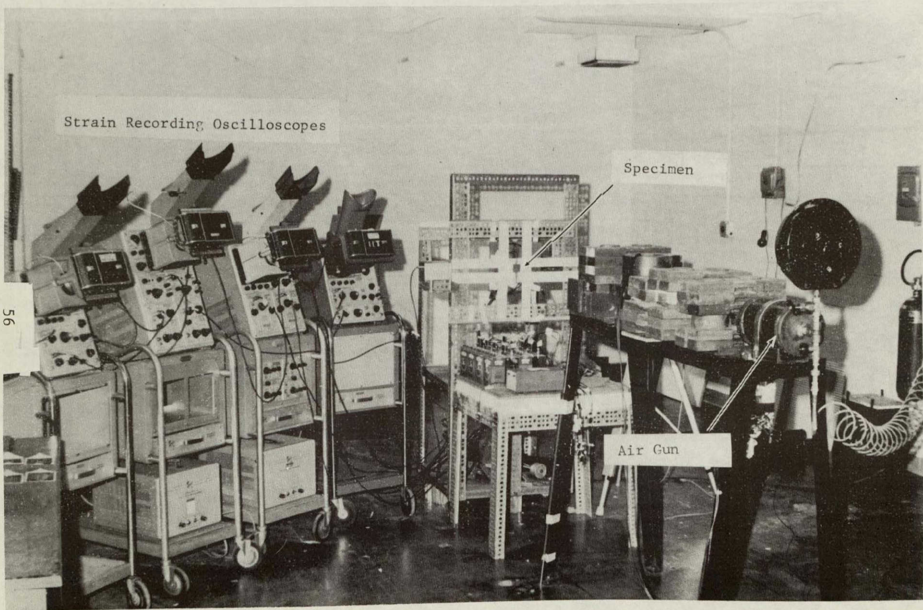
Fig. 9 EXPERIMENTAL SETUP FOR IMPACTING COMPOSITE PLATES AND RECORDING INSTRUMENTATION
