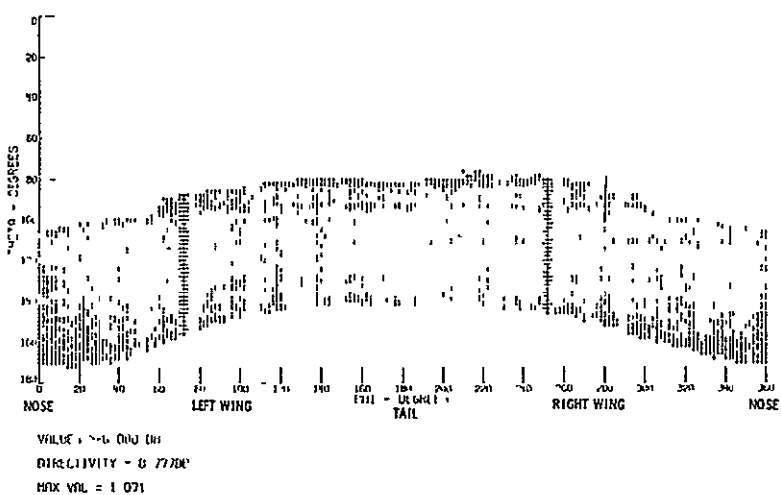
(p) Horizontally polarized coaxial fed slot antenna at station 950 on bottom fuselage.
