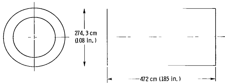
(a) Single rim. Material, Thornel/epoxy; rim diameter, 2.74 meters (9 ft); height, 4.72 meters (15 1/2 ft); total weight, 10 681 kilograms (23 548 lb); rotational speed, 6737 rpm.
