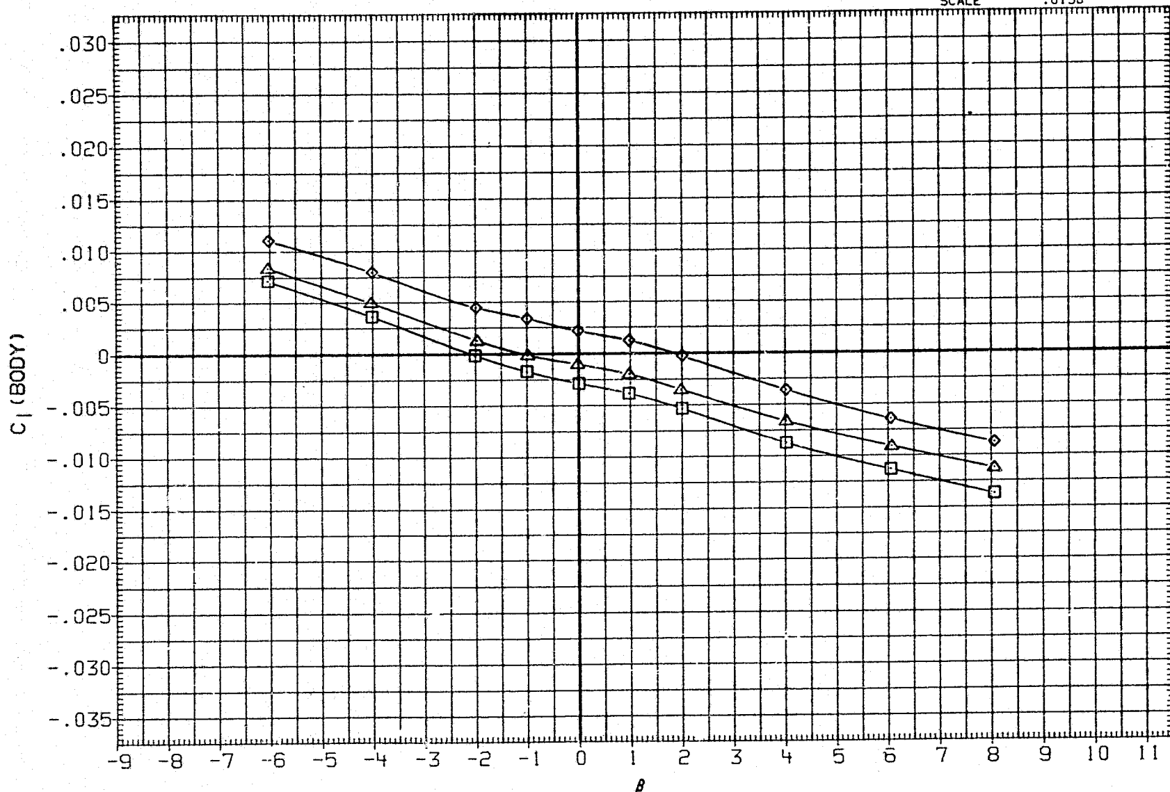
FIGURE 18(B). CONTROL SURFACE INTERACTION EFFECTS OF ELEVON,AILERON AND RUDDER DEFLECTION ON YAW POLARS,SPEED BRAKE AT 52.7 DEG.,ALPHA= 12 DEG.
