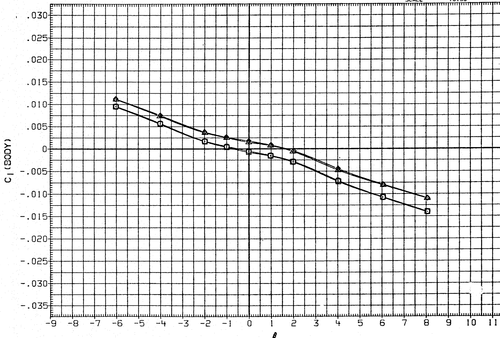
FIGURE 20. CONTROL SURFACE INTERACTION EFFECTS OF ELEVON,AILERON AND RUDDER DEFLECTION ON YAW POLARS,SPEED BRAKE AT 82.5 DEG.,ALPHA= 20 DEG.
