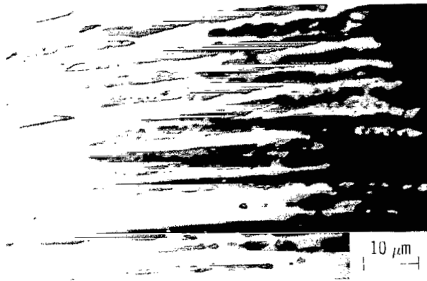
Figure 8. - Effect of 1800 thermal cycles (1100° to 425° C at 3-min intervals) on microstructure of directionally solidified eutectic alloy Fe-25Ta-22Ni-10Cr.
