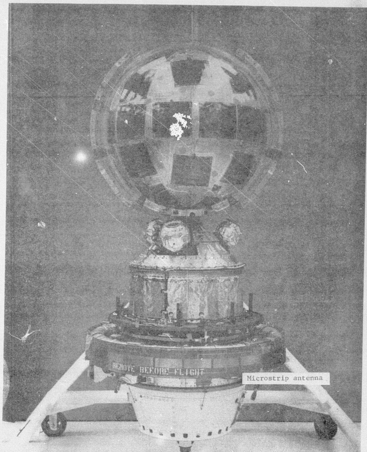
Figure 27. - Photograph of the S-band microstrip array on the Dual Air Density Satellite 24-element microstrip array (37-inch diameter).
