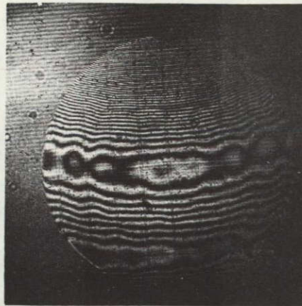
(a) Results obtained using Maksutov test without CGH
