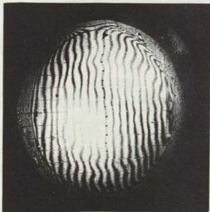
(c) Results obtained using null lens ( \lambda = 6328 \text{ \AA} )
